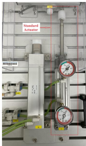
Figure 5.1 Standard Actuator with 32mm diameter and 100mm stroke cylinder.
