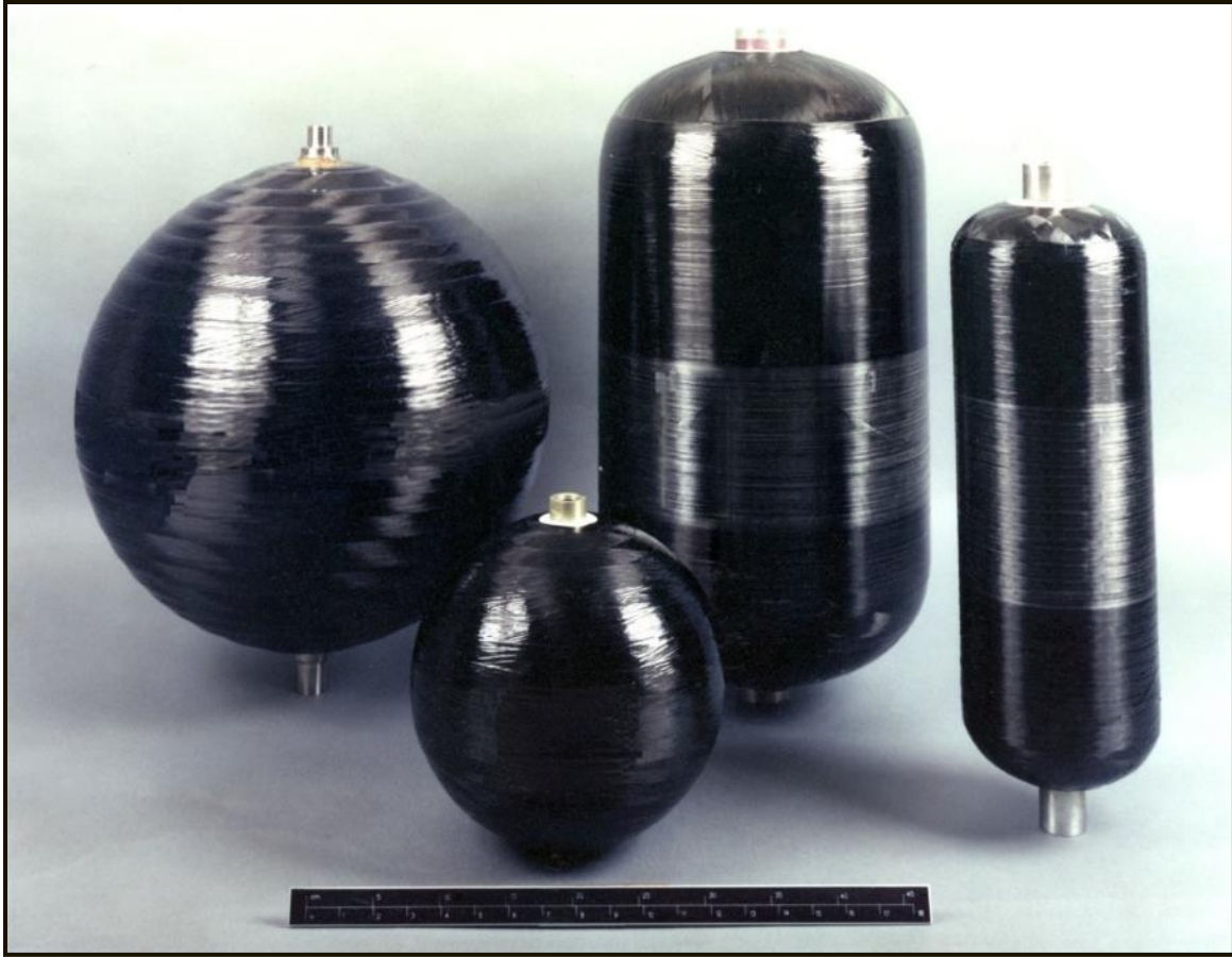
Figure 2.4 COPV manufactured by FW shown in different configurations [5]
