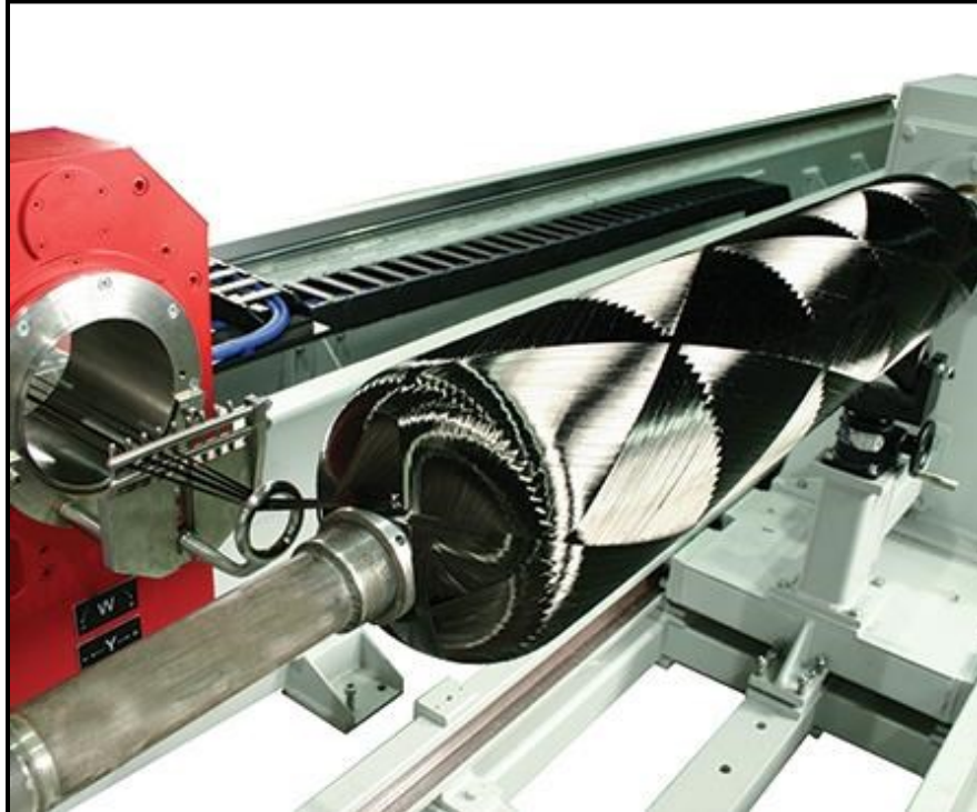
Figure 2.3 COPV manufactured by FW [5]
