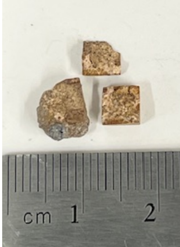
Figure 6.12 Si Alloy after one week of cyclic oxidation at 1000°C
