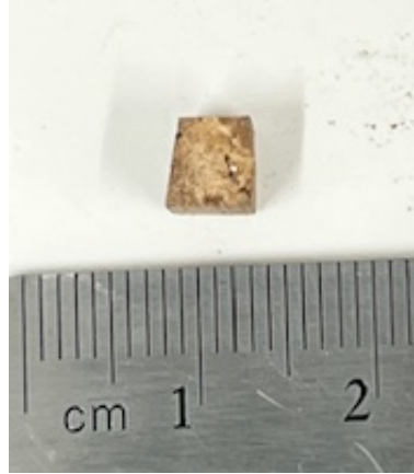
Figure 5.25 Si alloy after 48 hour static oxidation at 1000°C
