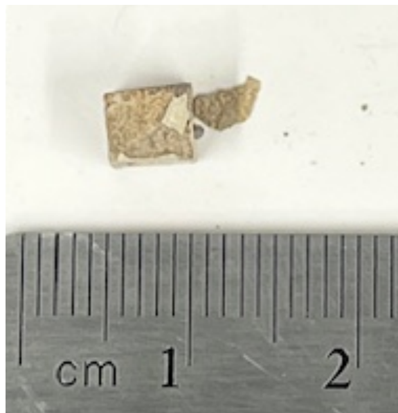
Figure 5.38 Si alloy after 72 hour static oxidation at 1000°C
