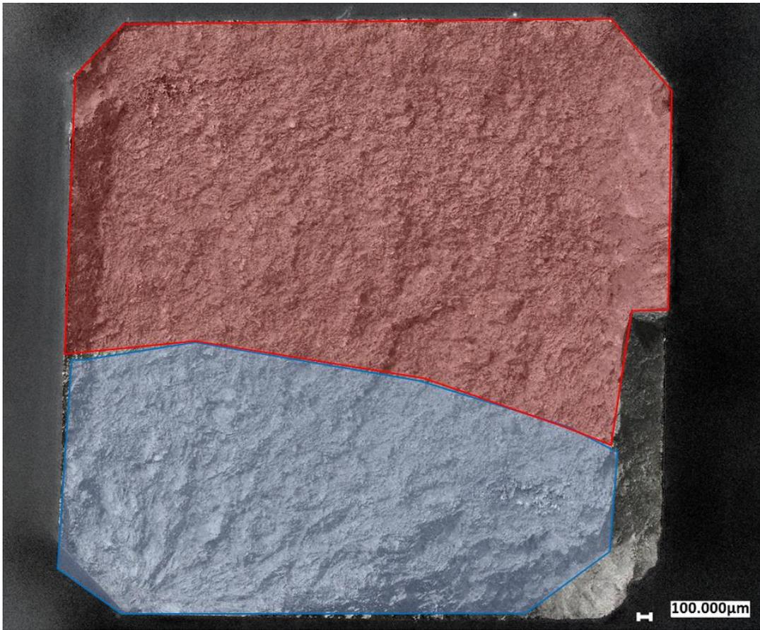
Figure 3.9 F49 (Polished)- Initiation site on the lower left side chamfer
