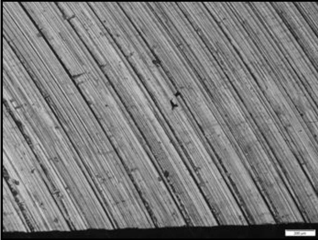
Figure 2.5 Milled specimen surface
