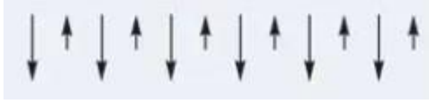
Figure 8: Diagram above demonstrates the orientation and magnitude of a ferrimagnetic material.
