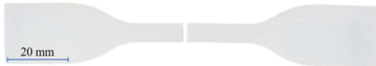
Figure 1.11: Typical Failure Mode of Durable Resin Tensile Specimens Tested at AT
