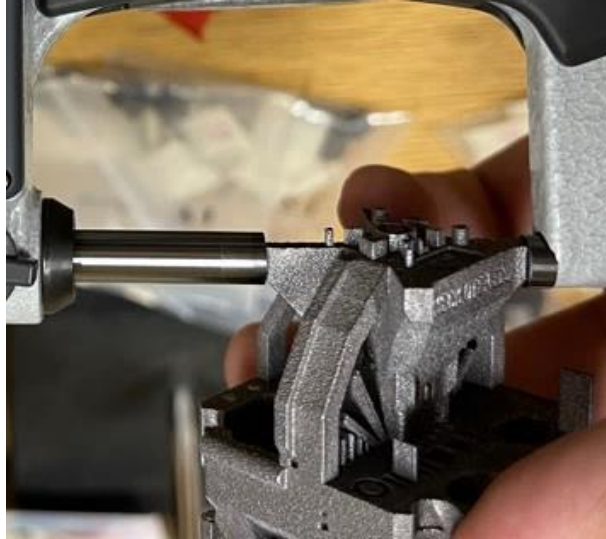
Figure 7 Feature measured by the micrometer method.
