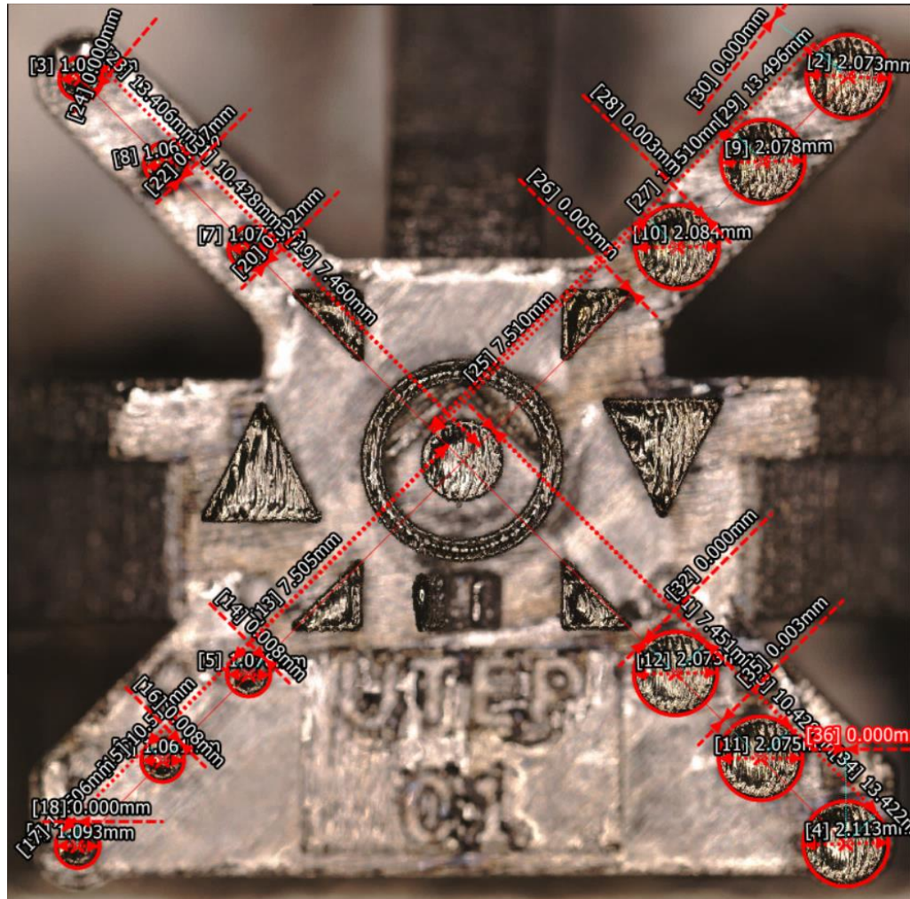
Figure 8 2D Plane measurement by an optical method.
