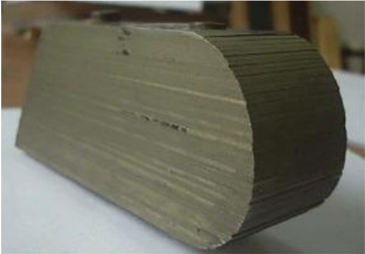
Figure 9 A sheet lamination component was produced and the layers are clearly visible upon completion [32].
