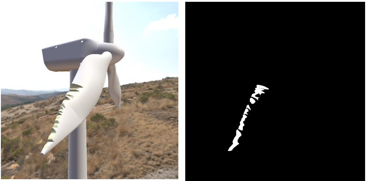
Figure 10 Leading Edge Erosion Image and Its Perspective Semantic Segmentation
