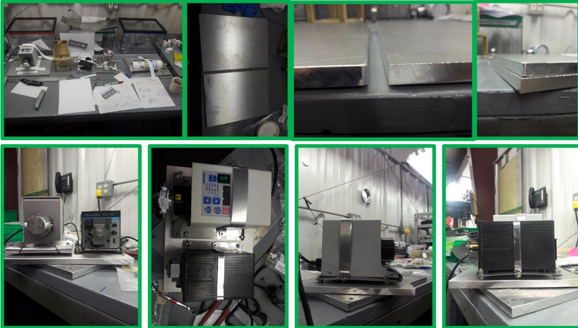
Figure 1.2. Designed, cut, and ended aluminum and stainless-steel supports, rails, and braces to belt devices and artefacts within the eml-II.
