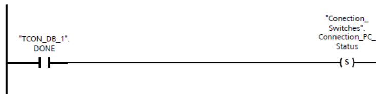
Figure 2.9: Network 2 (PLC-1) Indicates a successful connection with the admin PC.
