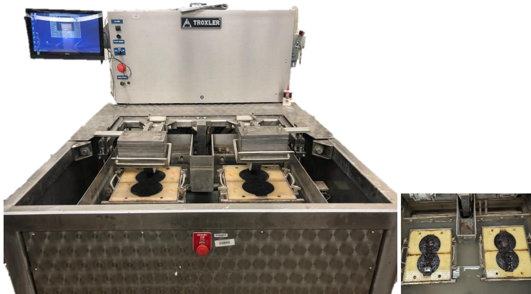
Figure 4.6. HWT Device and Specimen Setup
