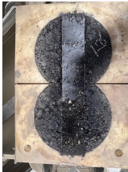
Figure 3.4. Condition of New mix after rutting test
