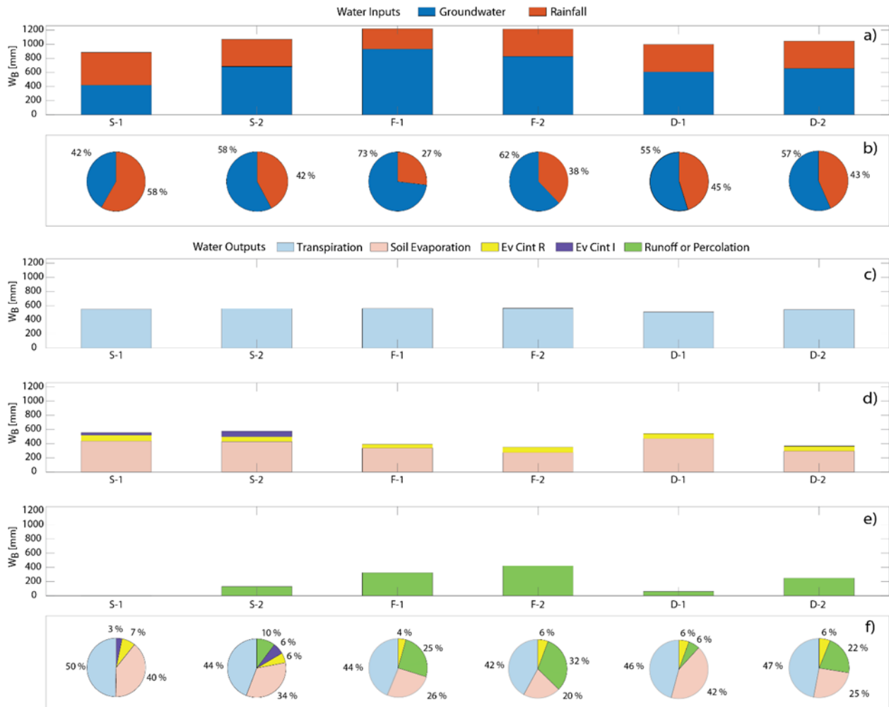
Figure 3.11 Water balance in the observation plots. a) main water inputs (red color is rainwater and blue is groundwater); b) water input proportion (in %) of rainwater and groundwater; c) use of water by the transpiration component; d) outflow of water from the system due to soil evaporation (light orange), evaporation of rainwater intercepted by the canopy (yellow), and evaporation of irrigation water intercepted by the canopy (purple color); e) runoff or percolation; f) proportion of water outputs (in %) by each component.
