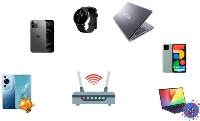
Figure 6.1: Many devices in an airport public Wi-Fi with a malicious attacker logged in, planning to exploit the devices on the network with a complex vulnerability (on the bottom right) and the decoy device placed by the defender trying to capture the attacker’s exploit (bottom left)
