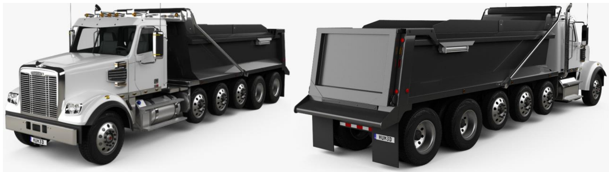
Figure 7.3: 3-D representation of an aggregate haul truck featuring the same axle configuration as the vehicle used at the road test in Virginia. Source: Hum3D.
