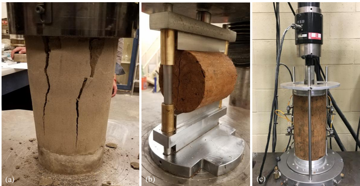
Figure 3.4: (a) UCS, (b) IDT strength, and (c) submaximal modulus laboratory testing apparatus.
