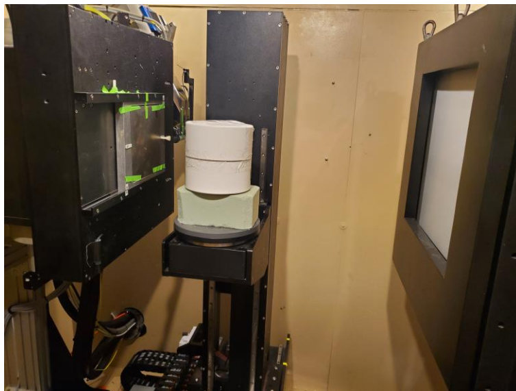
Figure 3.5: X-ray CT system used to analyze the cylindrical samples placed inside sealed PVC pipe caps used for protecting specimens during transport to the testing facilities.
