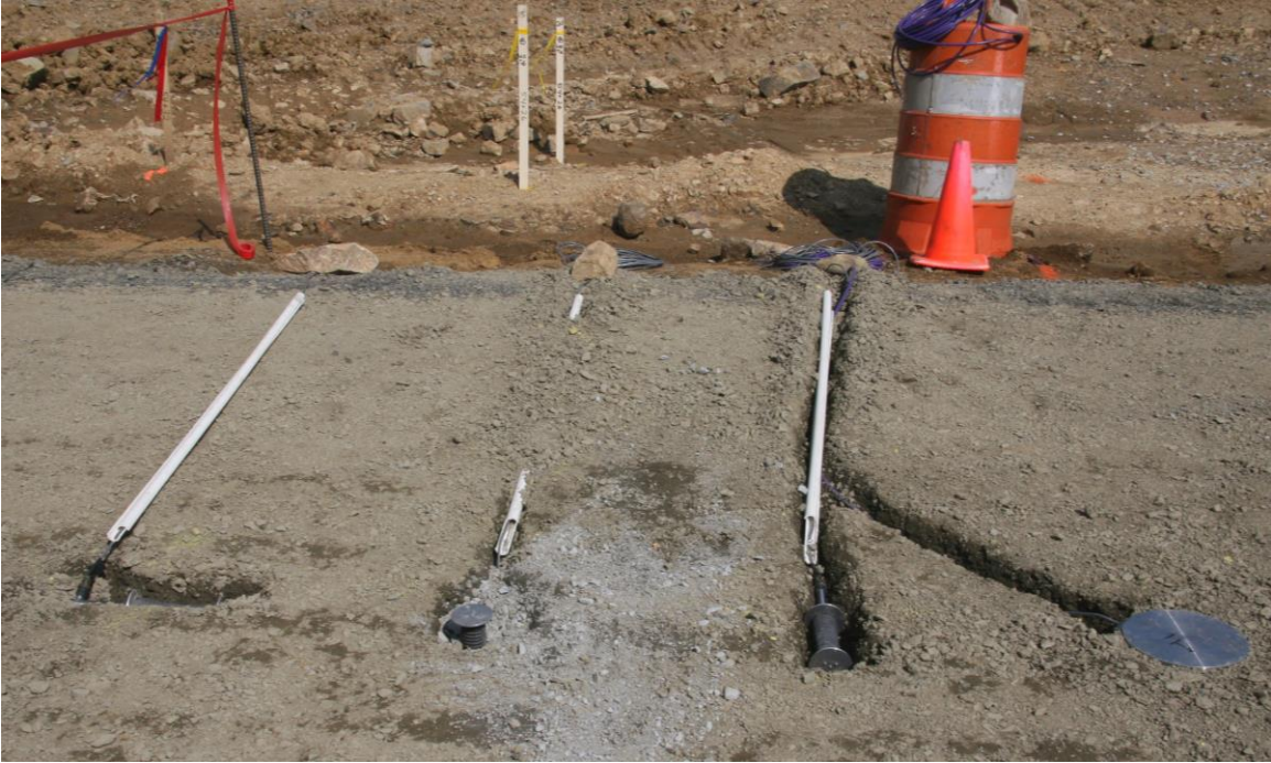
Figure 6.8: Longitudinal, transversal, and vertical LVDTs installed at the bottom of the UAB layer next to a pressure cell at the Virginia inverted pavement section.
