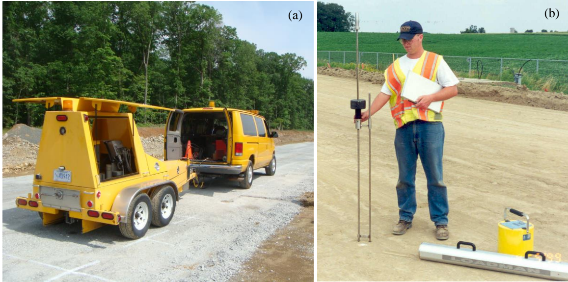
Figure 6.3: Falling Weight Deflectometer (a) and Dynamic Cone Penetrometer (b) used for in-site evaluation of the pavement structures at Bull Run Route 659.
