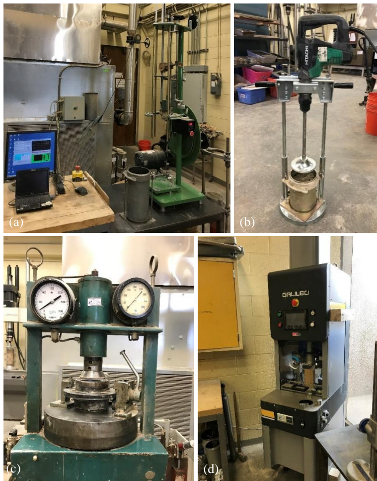
Figure 3.3: (a) Impact hammer, (b) vibratory hammer, (c) Texas Gyrotory Compactor, and (d) SuperPave Gyrotory Compactor used for compaction in the laboratory.
