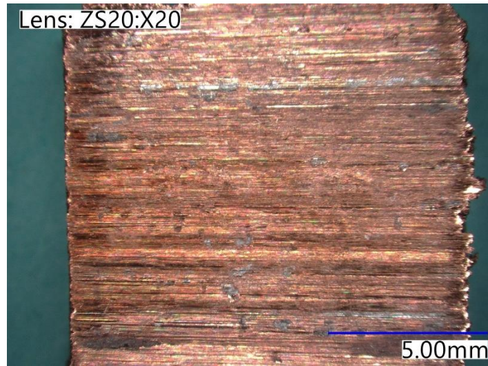
Figure 2.9. Digital optical microscope image at 20X magnification of a cross-section of the sintered part.
