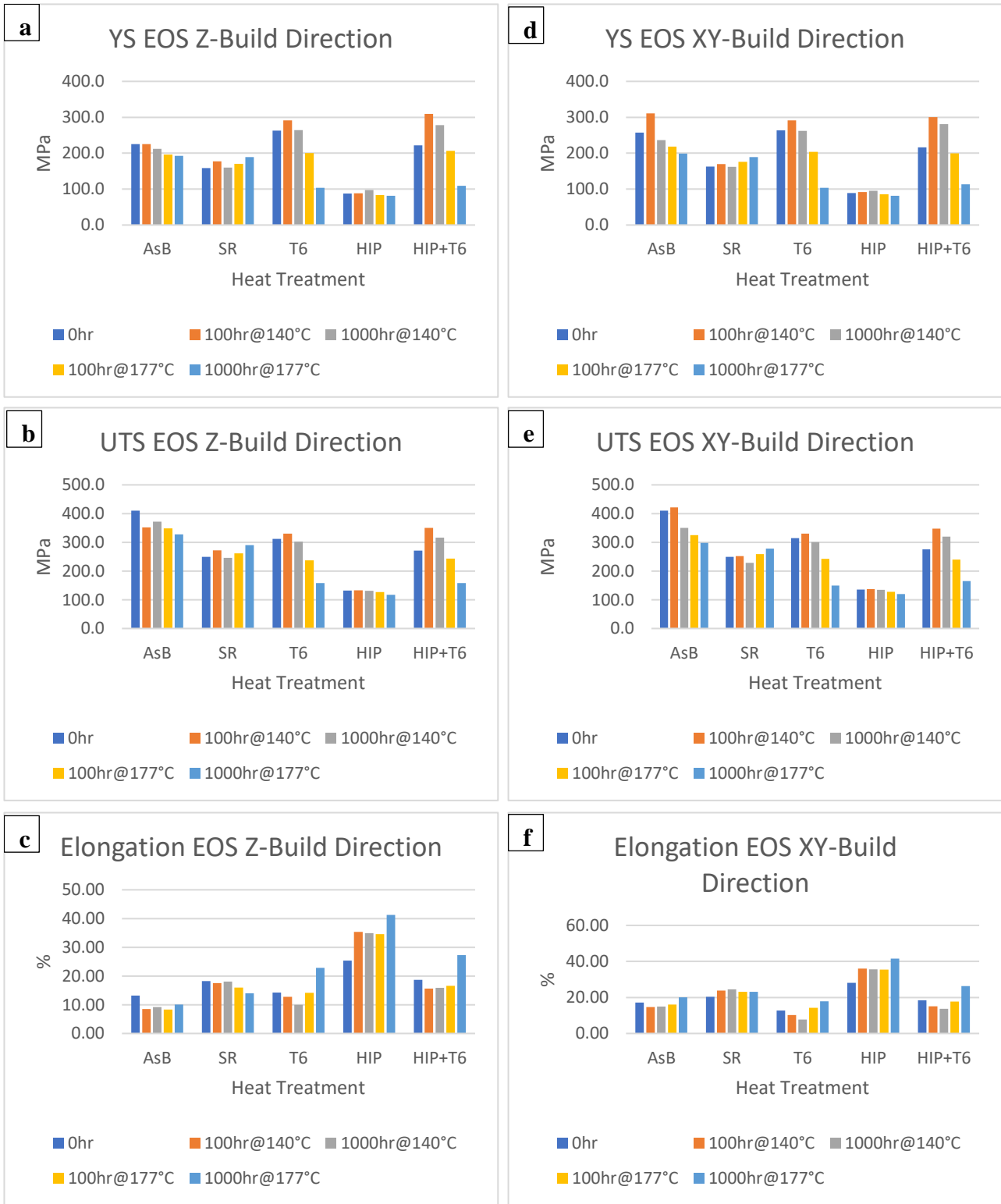
Figure 42. Comparative bar graphs showing mechanical properties for F37 on EOS printer, under different aging conditions for the different heat treatments and built in Z and XY orientation, a), d) Yield strength, b), e) UTS and c), f) Elongation; notice strength decreases with aging in a), b), d) and e), while elongation increases in c) and f) for T6, HIP and HIP+T6.
