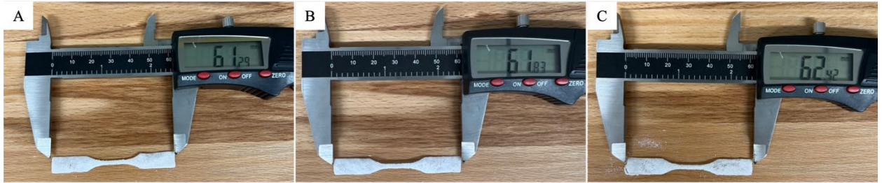
Figure 3.2: LS printed HDPE single-layer tensile specimens. Specimen 1 (A), Specimen 2 (B), and Specimen 3 (C).
