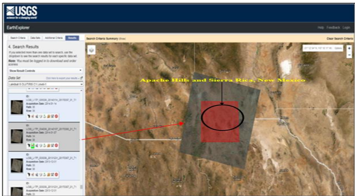
Figure 28: An image containing a geographical user interface created using the USGS Earth Explorer website. The red polygon & black circle shows the desired user-selected region; the grey area is the dataset results contained in the USGS data base for Landsat 8 (OLI) for the study area of the Apache Hills-Sierra Rica, New Mexico. The search results render various data sets. The data set (red arrow) used is LC08_L1TP_034038_20140107_20170306_01_T1 (Figure 21).
