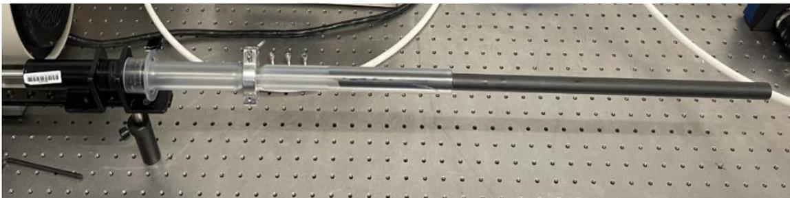
**Figure 3.19** Pyrometer optic/SiC tube fixture affixed to optic
