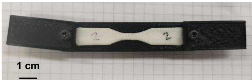
Figure 2.4: Fixture to recover sample.
