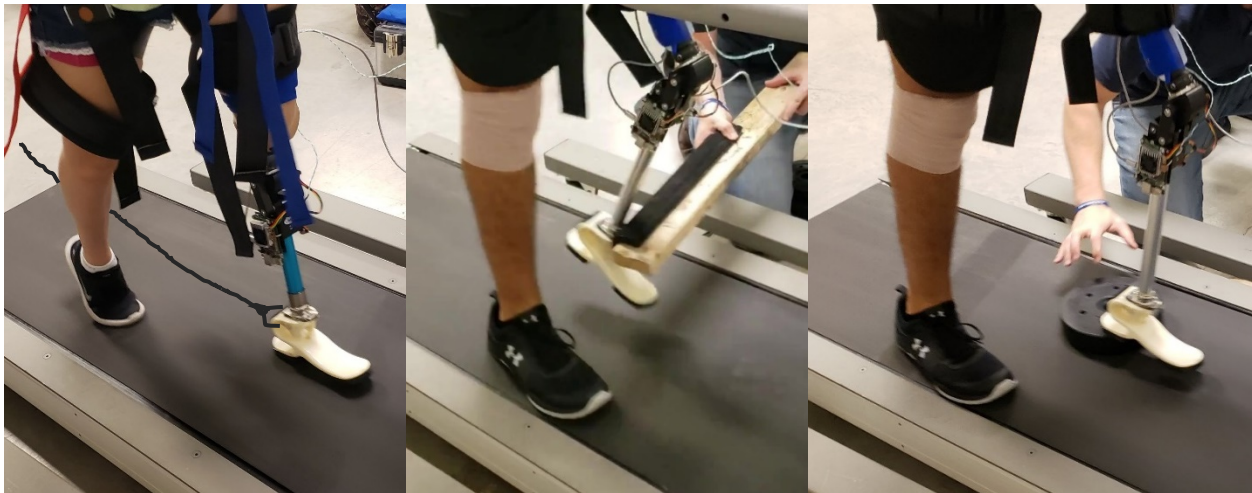
Figure 4.8: Examples of stumble induction for Subject 4 for stumble with bungee (left), obstacle (middle), and stumble with uneven ground (right). Leftmost image, demonstrating stumble with a bungee, is a simulated image showing the attachment point.
