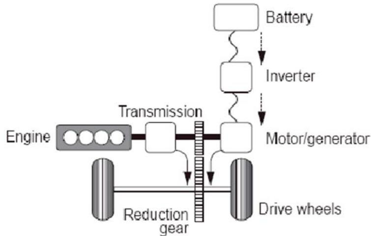
Figure 1.8: Parallel HEV configuration (Fayyad et al., 2012).
