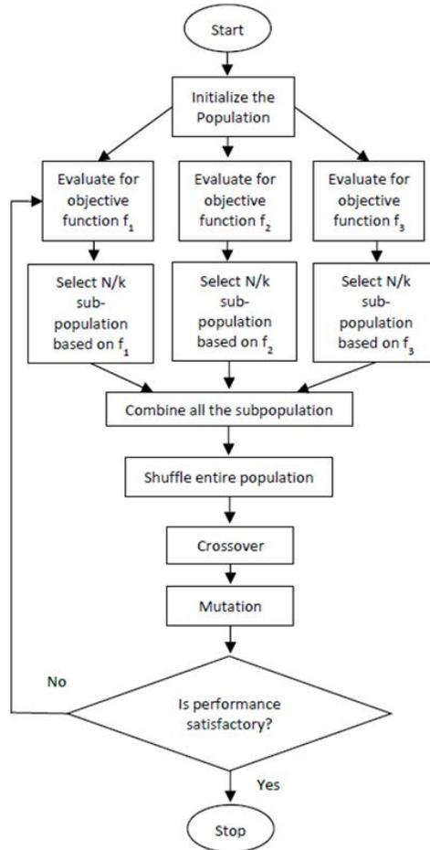
Figure 3.5: Schematic of VEGA's (Coello et al., 2007).
