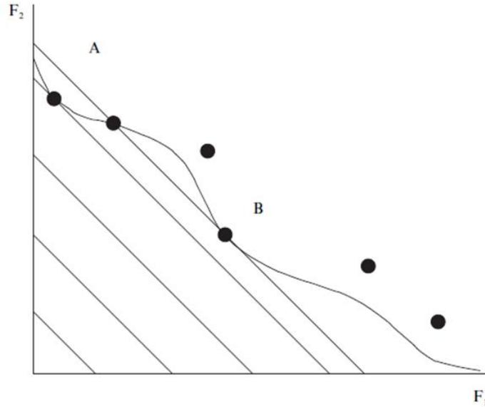
Figure 3.3: Priors weight selection for a bi-objective example in linear aggregating technique,  $w_1x_1+w_2x_2$  (Coello et al., 2007).
