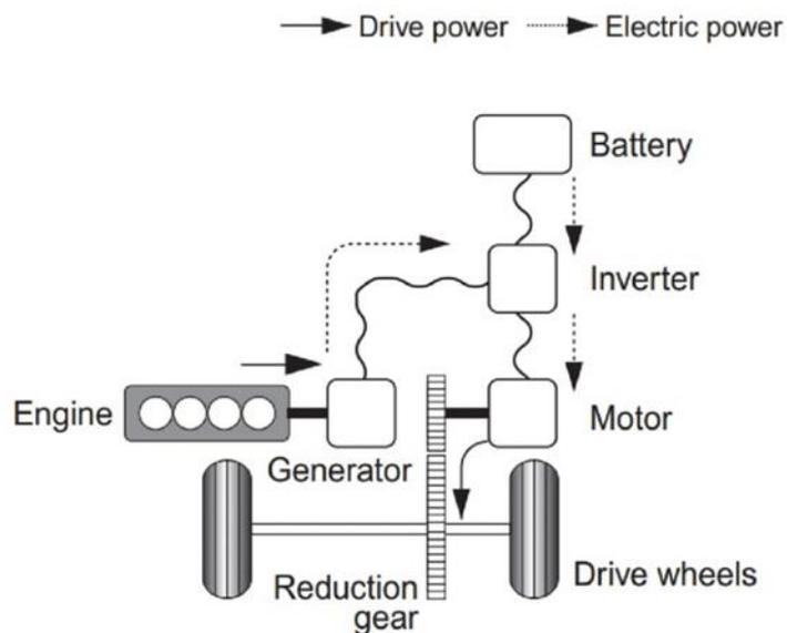
Figure 1.7. Series HEVs configuration (Fayyad et al., 2012).
