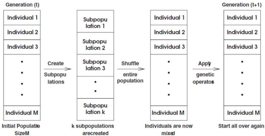
Figure 3.4: Schematic of VEGA’s selection mechanism.
