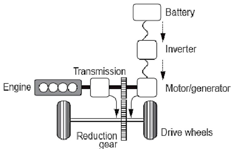
Figure 1.9: Series-parallel HEV configuration (Fayyad et al., 2012).
