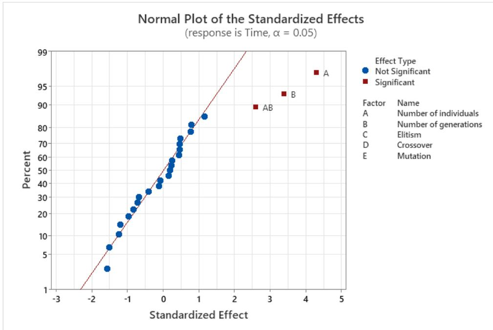
Figure 7.1: Normal plot of the effects for the normalized solution and computational time.
