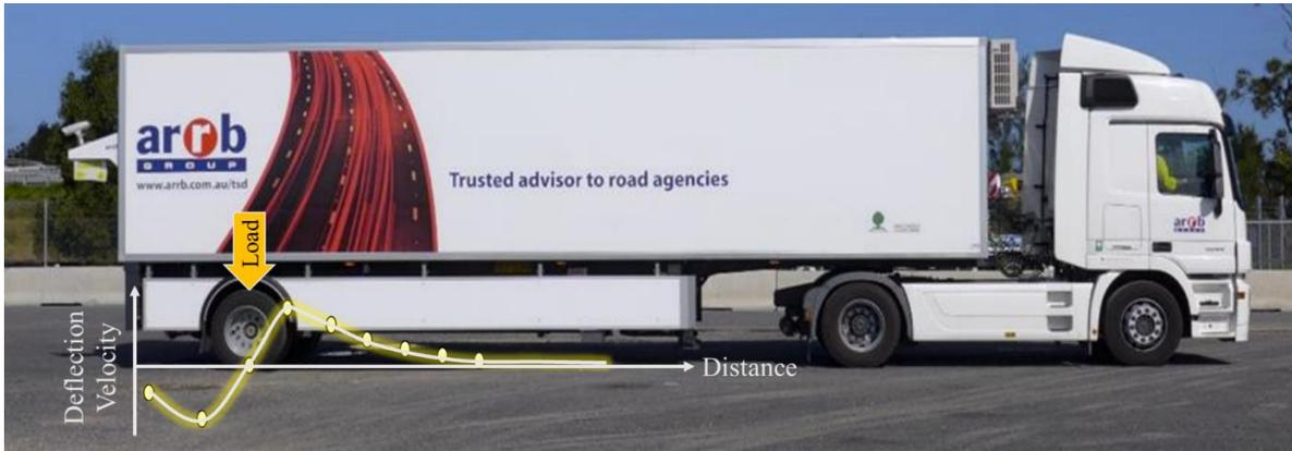
Figure 4.3: Australian Road Research Board (ARRB) TSD truck.
