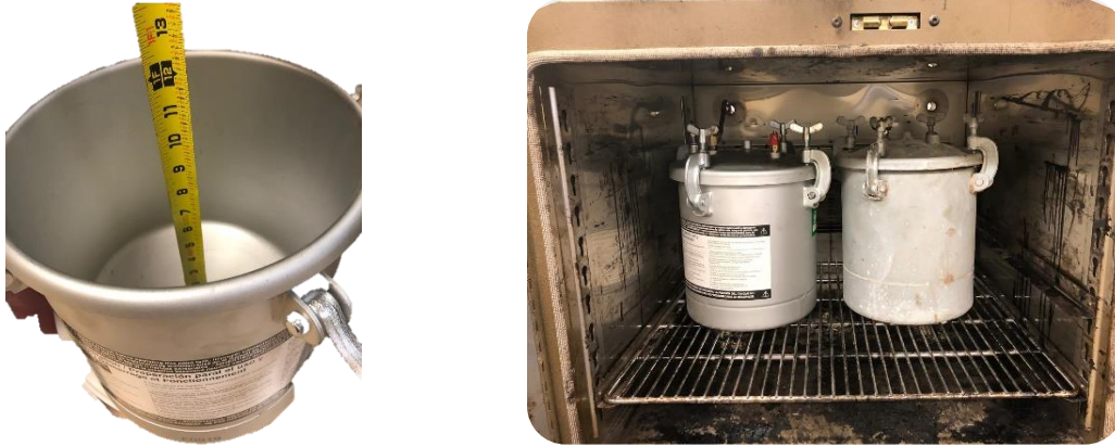
Figure 4.2. Pressure Aging Chamber for Loose Mix ( Protocol 3 )
