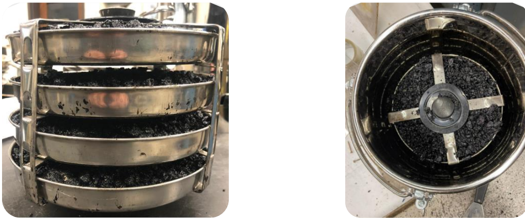
Figure 5.22. Stainless Steel Stand and Pressure Device Setup
