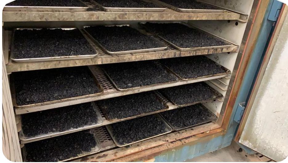
Figure 4.1. Loose Mixture Aging in Oven ( Protocol 1 and Protocol 2 )
