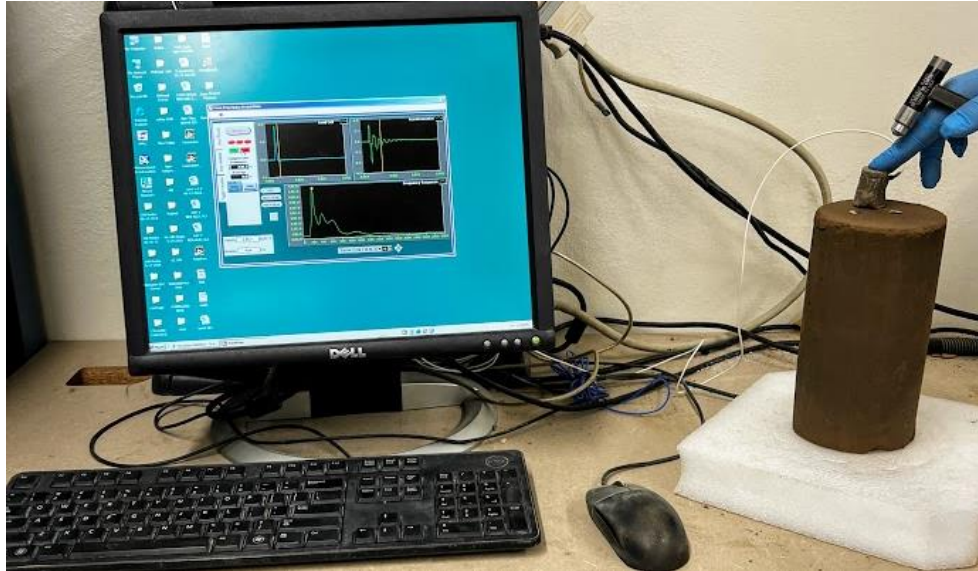
Figure 33: Free-Free Resonant Column Testing for Seismic Modulus
