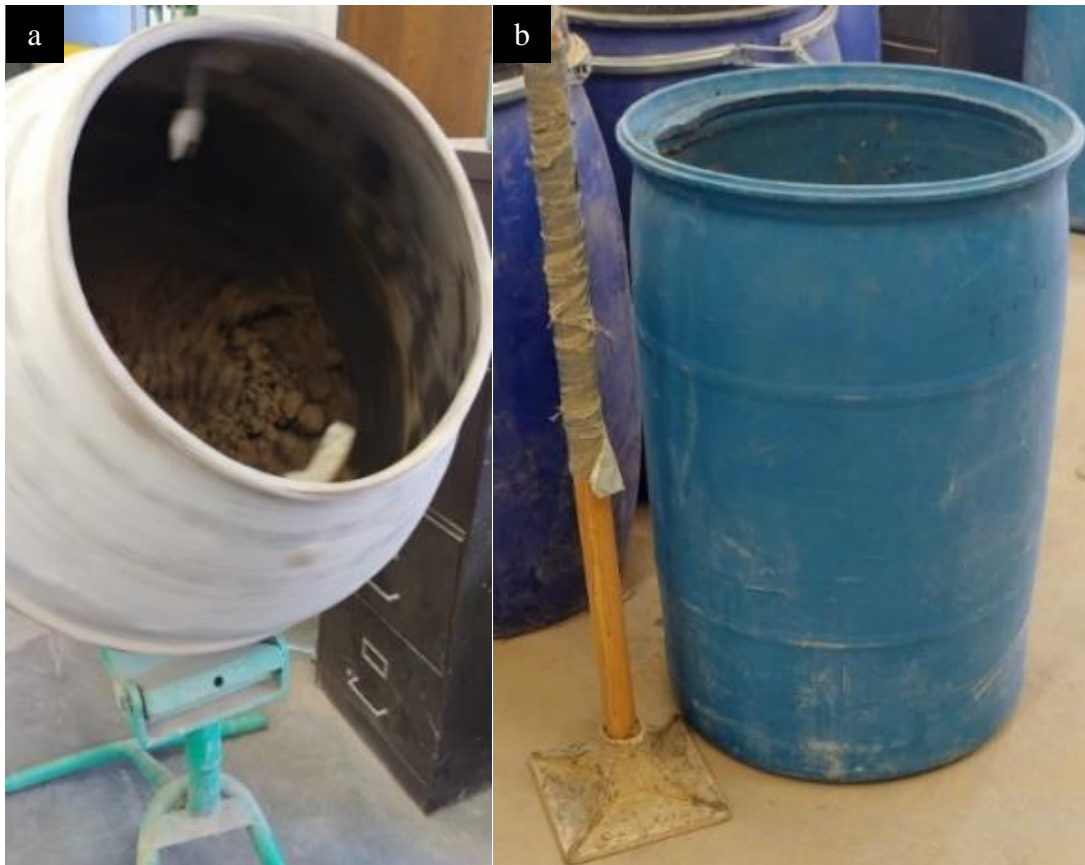
Figure 39: (a) Mixer and (b) Concrete Stamper with Barrel Used to Prepare Large Scale Specimens
