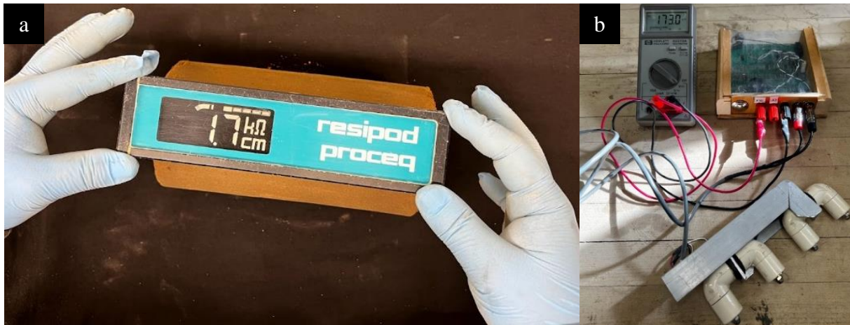
Figure 32: (a) Traditional Wenner Array (b) Laboratory-Created Array
