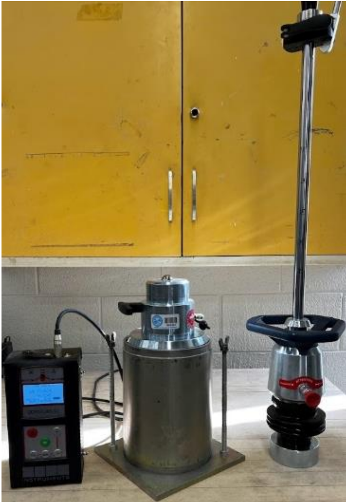
Figure 35: Lightweight Deflectometer Testing
