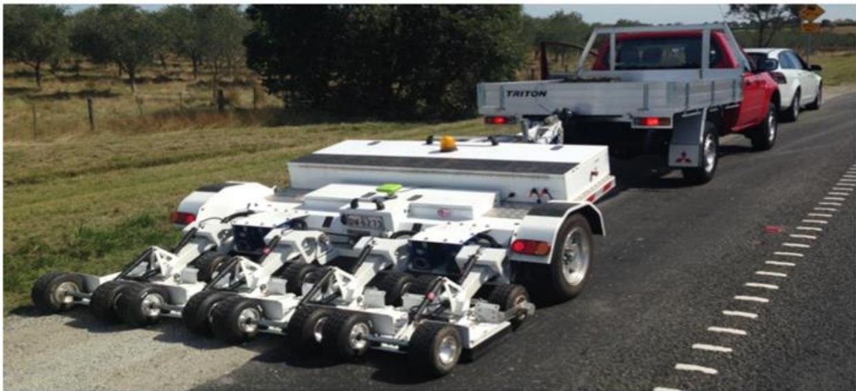
Figure 20: Second Generation NM-GPR System Incorporating a Traffic-Speed 3D Ground-Coupled Antenna Array
