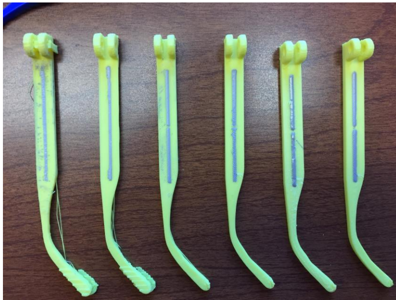
Figure 3.2 Print iterations of dipole antenna on an arm for a pair of glasses.
