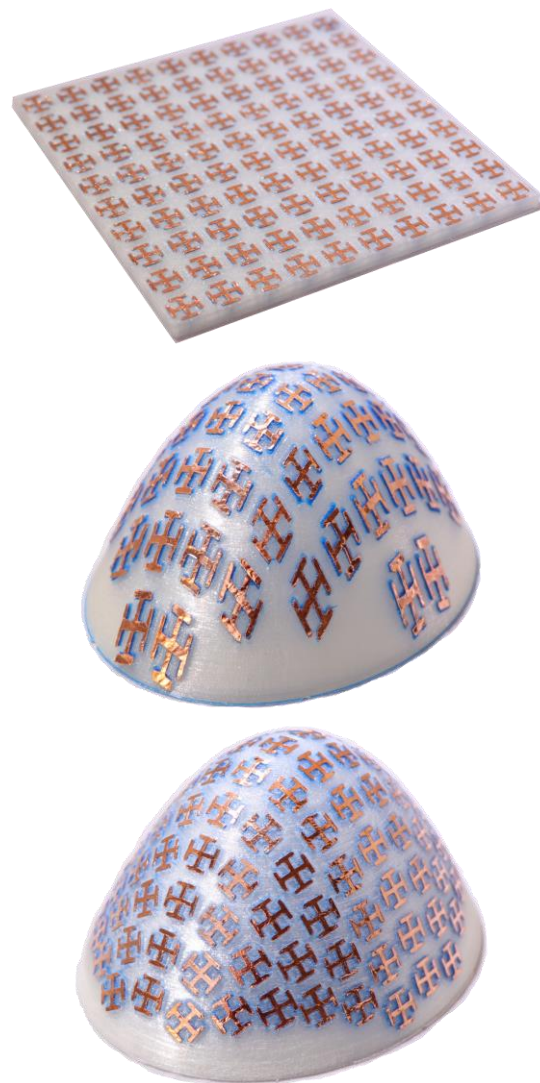
Figure 4.10 All three assembled FSS devices. From top to bottom, flat FSS, projected FSS, and conformal SVL FSS.
