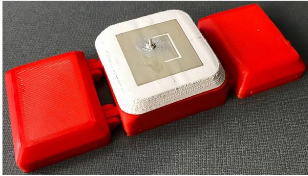
Figure 3.5 (Left) Final tested device featuring u-slot antenna on hi-k substrate atop of red PLA housing. (Right) Simulated and measured return loss.
