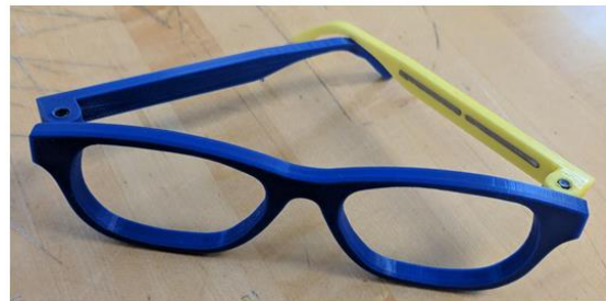
Figure 3.3 (Left) Return loss (S11) for two different feeding mechanisms. (Right) Complete set of eyeglasses, antenna arm shown in yellow.
