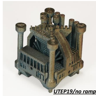
Figure 49 AconityMIDI+ fabricated UTEP18/ramp and UTEP 19/no ramp macro images post heat treatment
