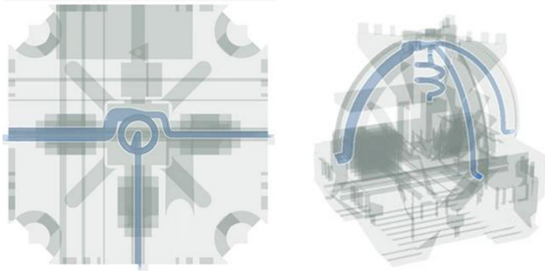
Figure 17 Wire view of test artifact highlighting the internal passageway utilized to test powder removal and surface finish/finishing of internal features.
