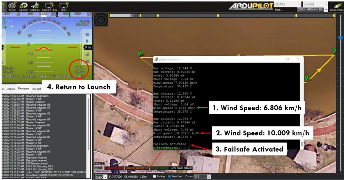
Figure 42. Base Station with Failsafe Command Activated.
