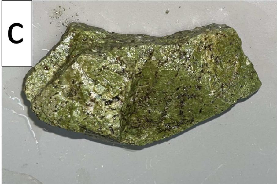
Figure 9c. Rock sample (c) is epidote. Collected from the SMD at Cottonwood Springs.
