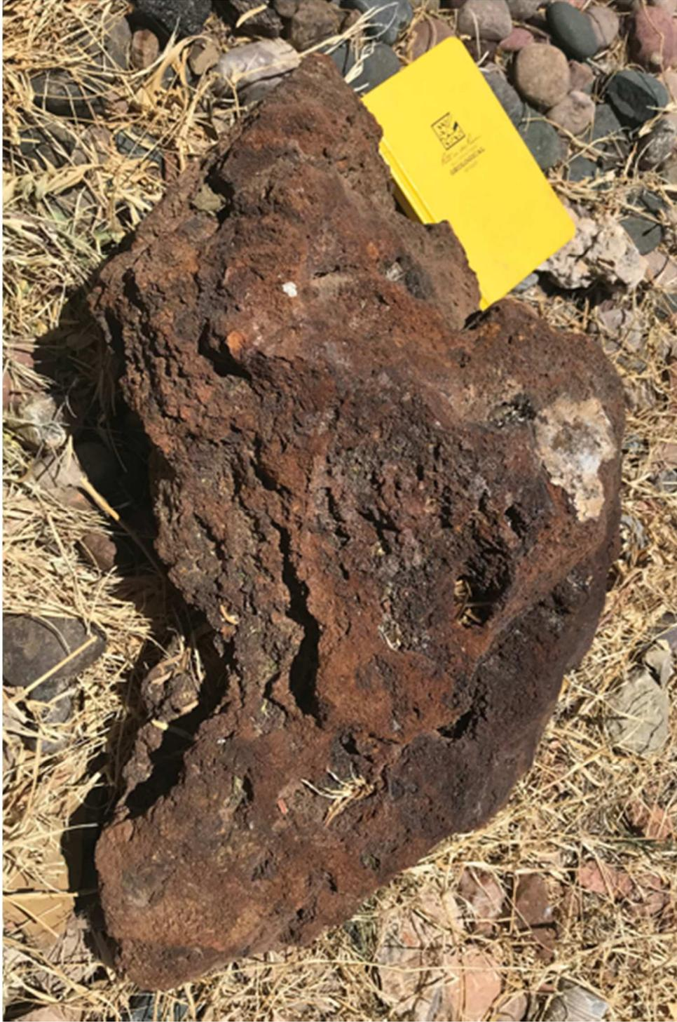
Figure 8. Sample of limonite gossan taken from outcrop 1 km /north of Cottonwood Springs as seen on Figure 1 green square.
