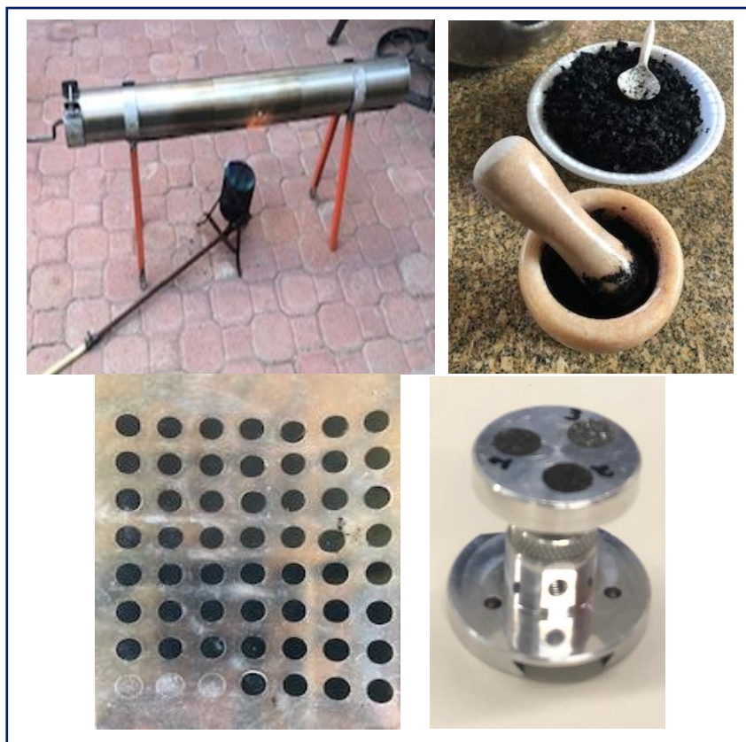
Illustration 6.1: Images of AC and carbon tape needed to place the sample under the SEM/EDS.
