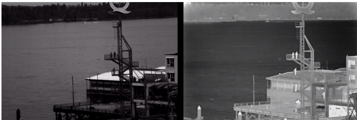
Figure 6.2: A Side-by-side Comparison of Near Infrared (NWIR) and Long Wave Thermal Infrared (LWIR) Cameras Display of a Scene [6].
