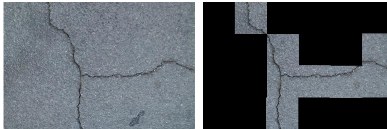
Figure 4.2: Input (Left) and Typical Output (Right) of a Deep Learning-based IC by Stacking Positive Class Patches [1]
