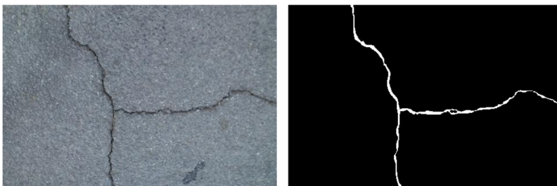
Figure 4.4: Input (Left) and Typical Output (Right) of a Deep Learning-based Semantic Segmentation (SS) [2]
