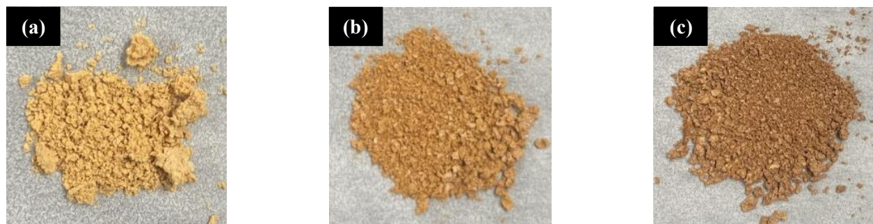
Fig. 4.8 – IBA products through SCS using glycine in a furnace: (a) 1:2 Fe/Al ratio, (b) 1:1 Fe/Al ratio, (c) 2:1 Fe/Al ratio.
