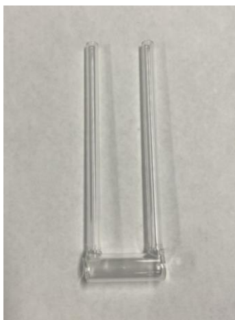
Fig. 3.8 – Empty sample cell where sample powder is placed inside.
