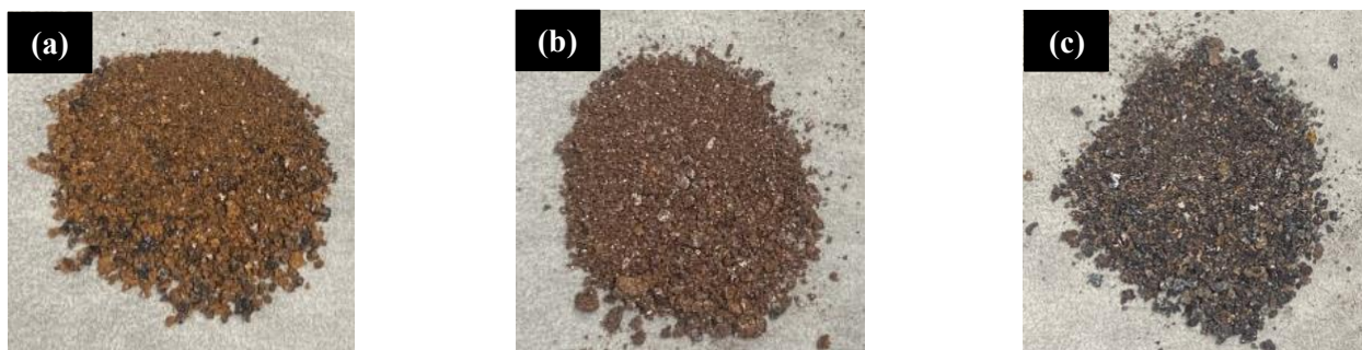
Fig. 4.5 – IBA products through SCS using citric acid on a hotplate: (a) 1:2 Fe/Al ratio, (b) 1:1 Fe/Al ratio, (c) 2:1 Fe/Al ratio.
