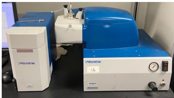
Fig. 3.6 – Microtrac Bluewave particle size analyzer (right) with sample delivery controller (left).
