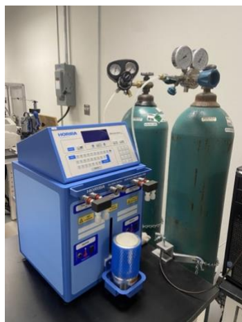
Fig. 3.7 – HORIBA SA 9600 BET Multipoint Surface Area Analyzer with secured helium and nitrogen tanks.
