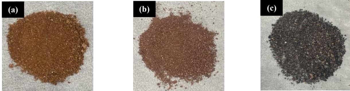
Fig. 4.6 – IBA products through SCS using citric acid in a furnace: (a) 1:2 Fe/Al ratio, (b) 1:1 Fe/Al ratio, (c) 2:1 Fe/Al ratio.
