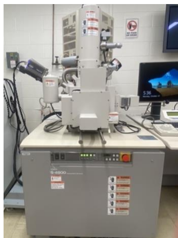
Fig. 3.3 – Hitachi S-4800 High Resolution SEM instrument.
