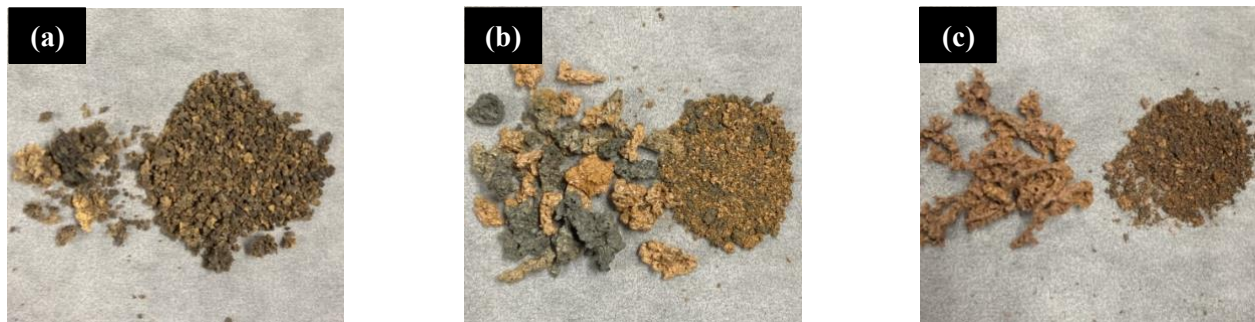
Fig. 4.7 – IBA products through SCS using glycine on a hotplate: (a) 1:2 Fe/Al ratio, (b) 1:1 Fe/Al ratio, (c) 2:1 Fe/Al ratio.
