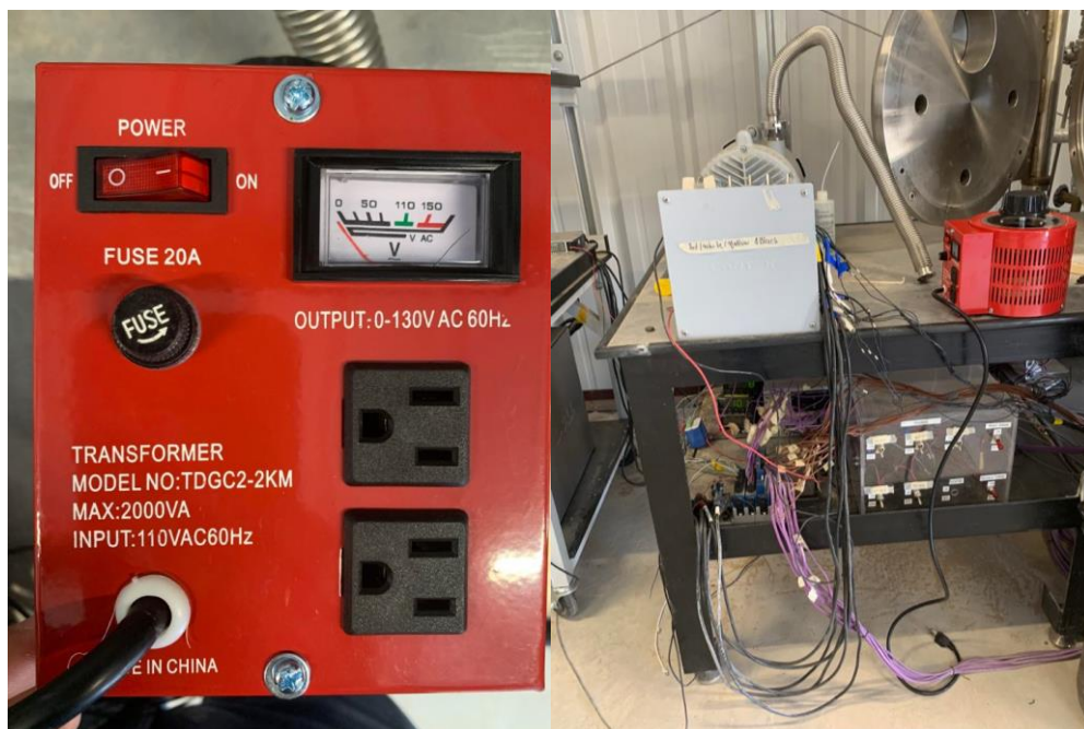
Figure 5-6. VARIAC, variable transformer
