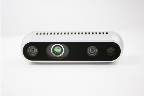
Figure 5.2: Intel RealSense D435i Depth Camera
