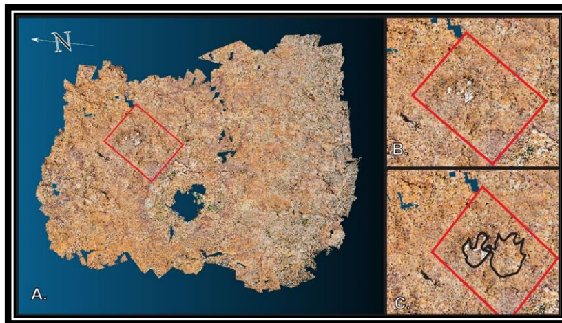
Figure 11- Dense point cloud model, HH_VM_Mega, based on the handheld camera data (Martinez, 2016). A. shows the entire surveyed area, B. is a closeup of one particularly prominent footprint with traces of plaster embedded, and C. shows an outline of the prominent footprint and an adjacent footprint that was identified from the model. The red box outlines the area of the 2 footprints and shown in figures throughout the paper.
