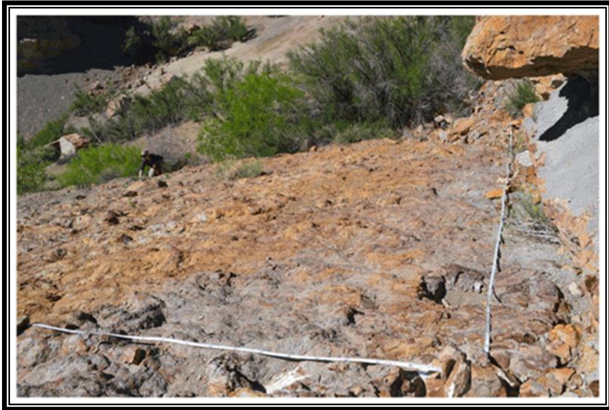
Figure 4- The grid system used in this study was based on two metric tape measures laid out perpendicular to each other to establish the locations for photographs. The positions of the individual grid intersections at 1 m spacing were marked as shown in Figure 2.5.
