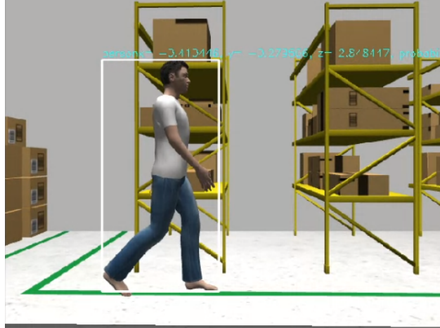
Figure 5.3: Object detection using the Deep Learning OpenCV framework and a pre-trained SSD MobileNet model
