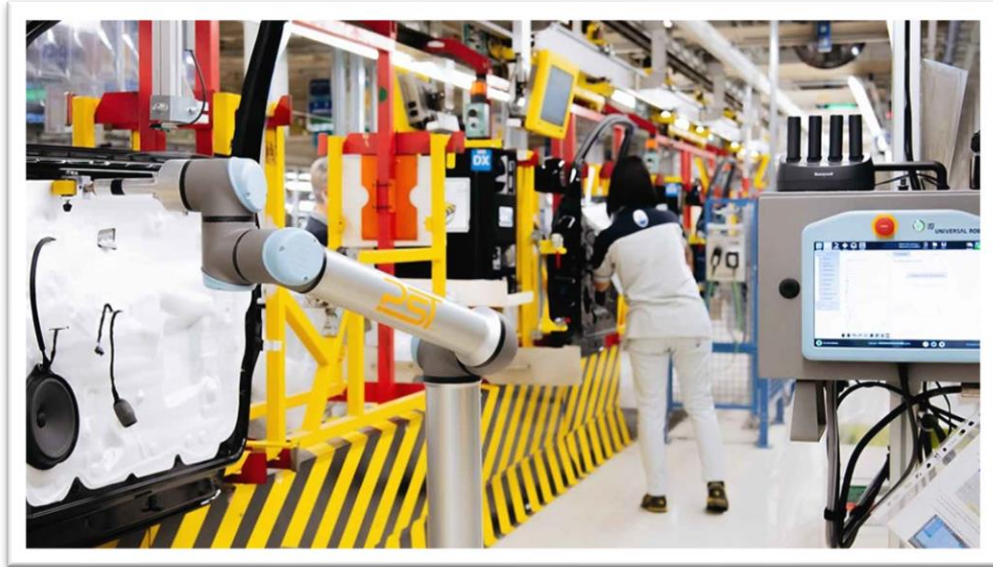
Figure 1.3.3: Universal Robot with a roller end-effector at Fiat (Stellantis) pressing seal tape on door panels [39]
