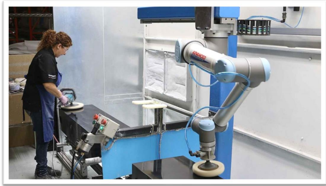
Figure 1.2.4: UR10 with polish pad end-effector working simultaneously with an operator at Paradigm
