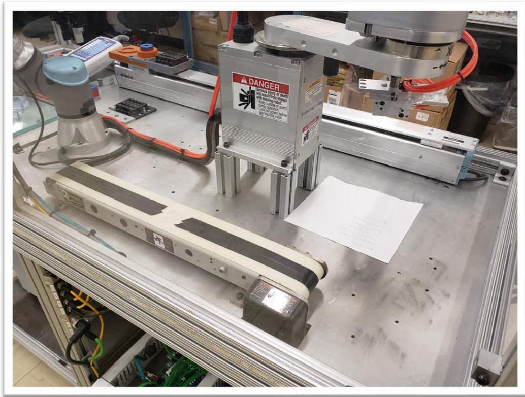
Figure 2.2.10: Linear actuator for failed assemblies
