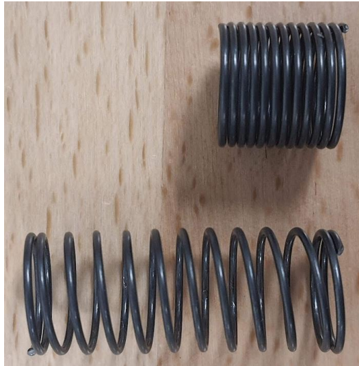
Nitinol Shape Memory Alloy Springs
