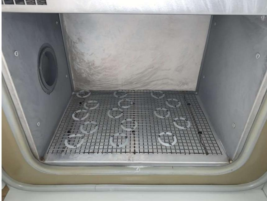
Figure 19: Gaskets in Tenney Environmental Chamber for Thermal Soak
