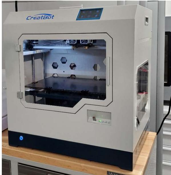
Figure 6 - Creatbot F430 FFF 3D Printer
