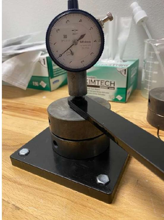
Figure 10: ASTM F38 Testing Assembly
