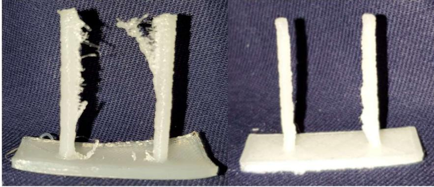
Figure 14: Retraction Test with (a) Stringing and (b) No Stringing
