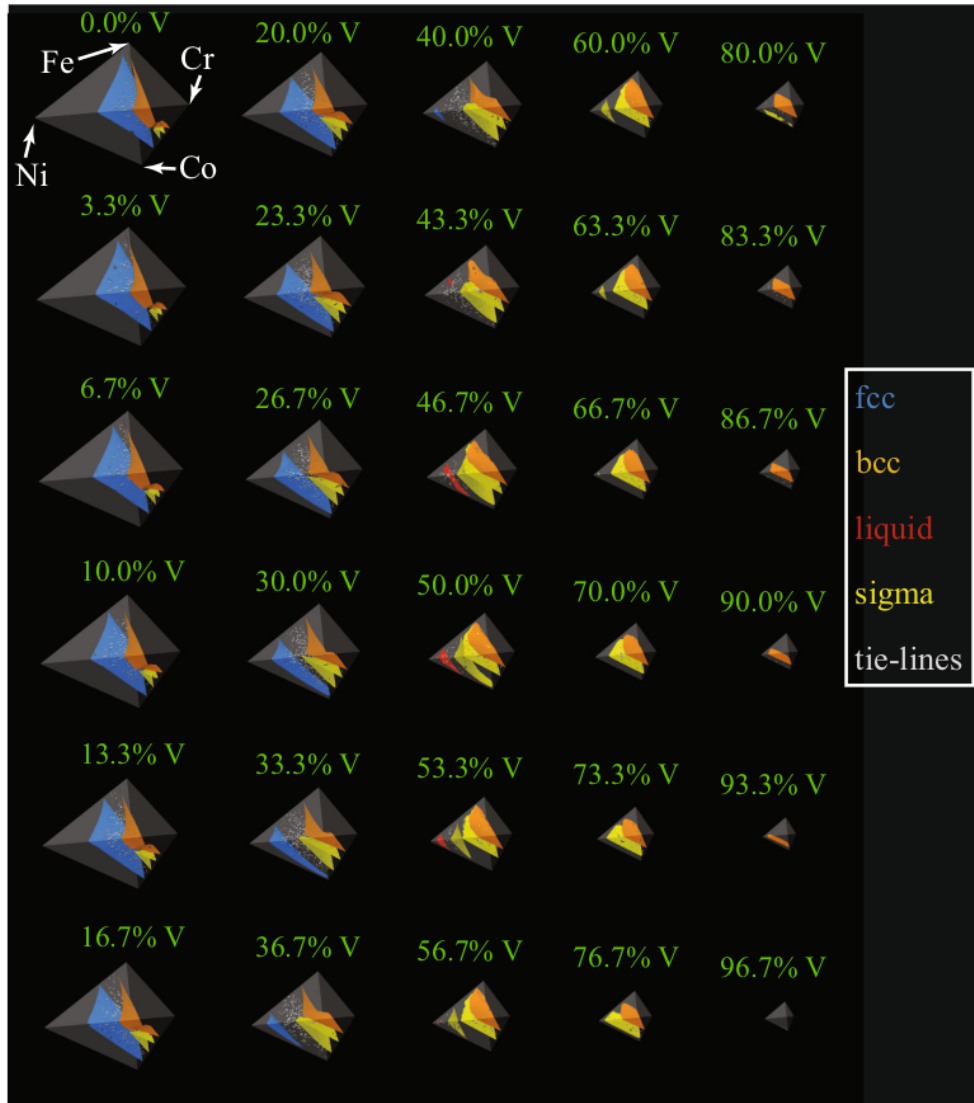
Figure 8.6: Co-Cr-Fe-Ni-V system where the surfaces indicate phase boundaries and the concentration of V is gradually increased from 0% to about 100% [12]
