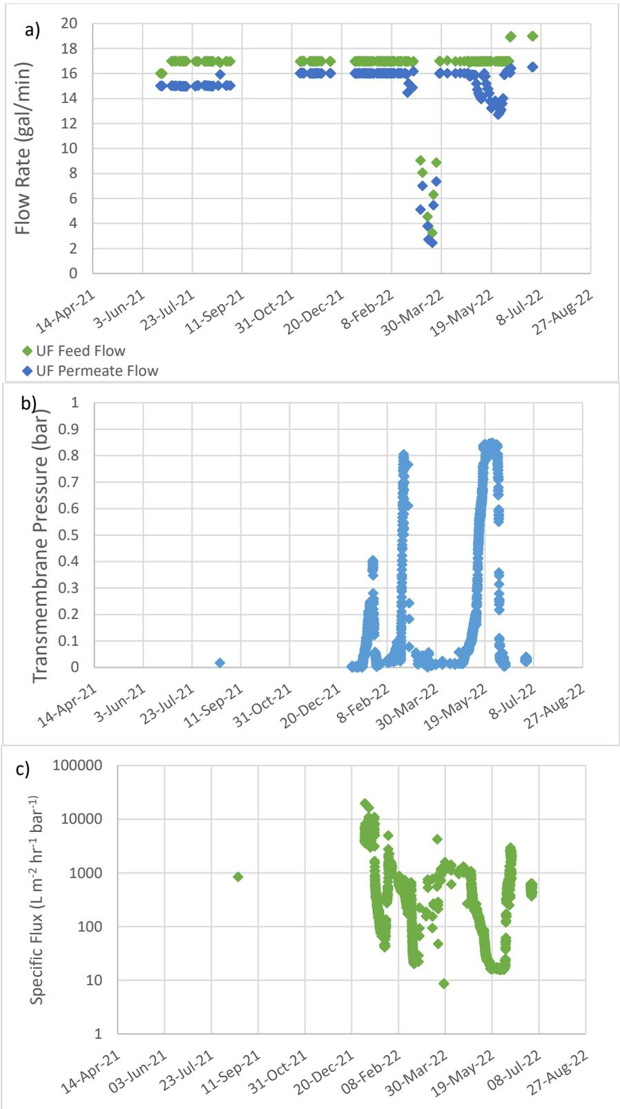
Figure 4. a) Daily Median for UF Feed and Permeate Flow, b) Hourly Median Transmembrane Pressure, and c) Hourly Median Specific Flux.
