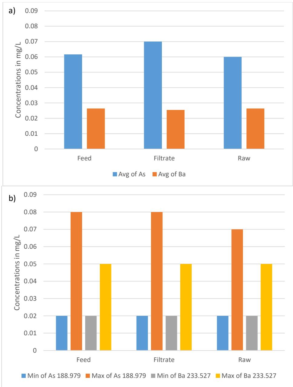
Figure 13. a) Average concentrations of As and Ba. b) Maximum and Minimum Concentrations of As and Ba
