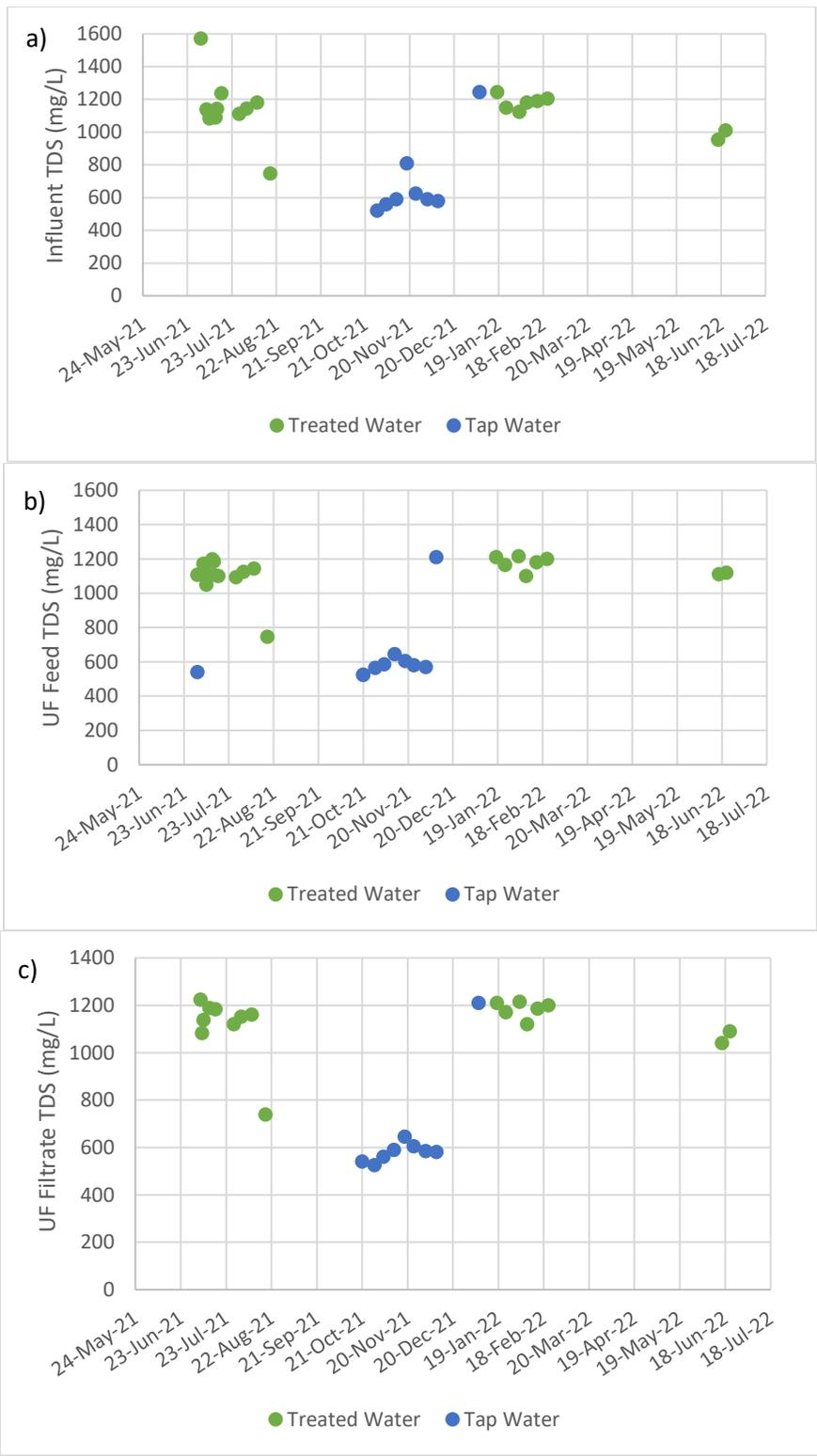
Figure 11. a) Influent TDS, b) UF Feed TDS, and c) Filtrate TDS (June 2021-June 2022)
