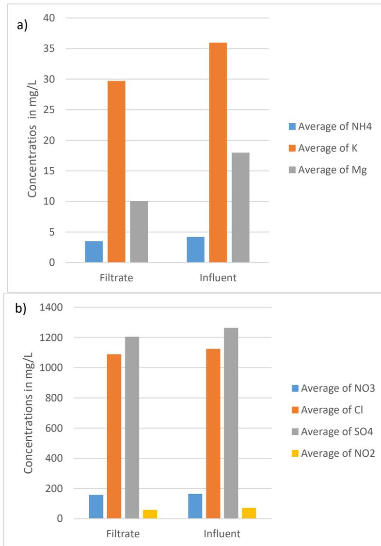
Figure 12. a) Average Concentrations of K,  $\text{NH}_4$  and Mg b) Average Concentrations of Cl,  $\text{SO}_4$ ,  $\text{NO}_3$  and  $\text{NO}_2$ .
