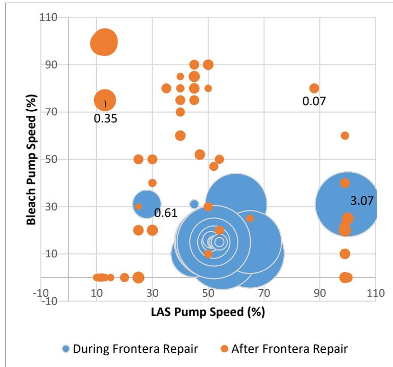
Figure 2. Monochloramine Concentrations (mg/L) in UF Feed Water versus chemical dosing pump speeds (August 2021- August 2022).
