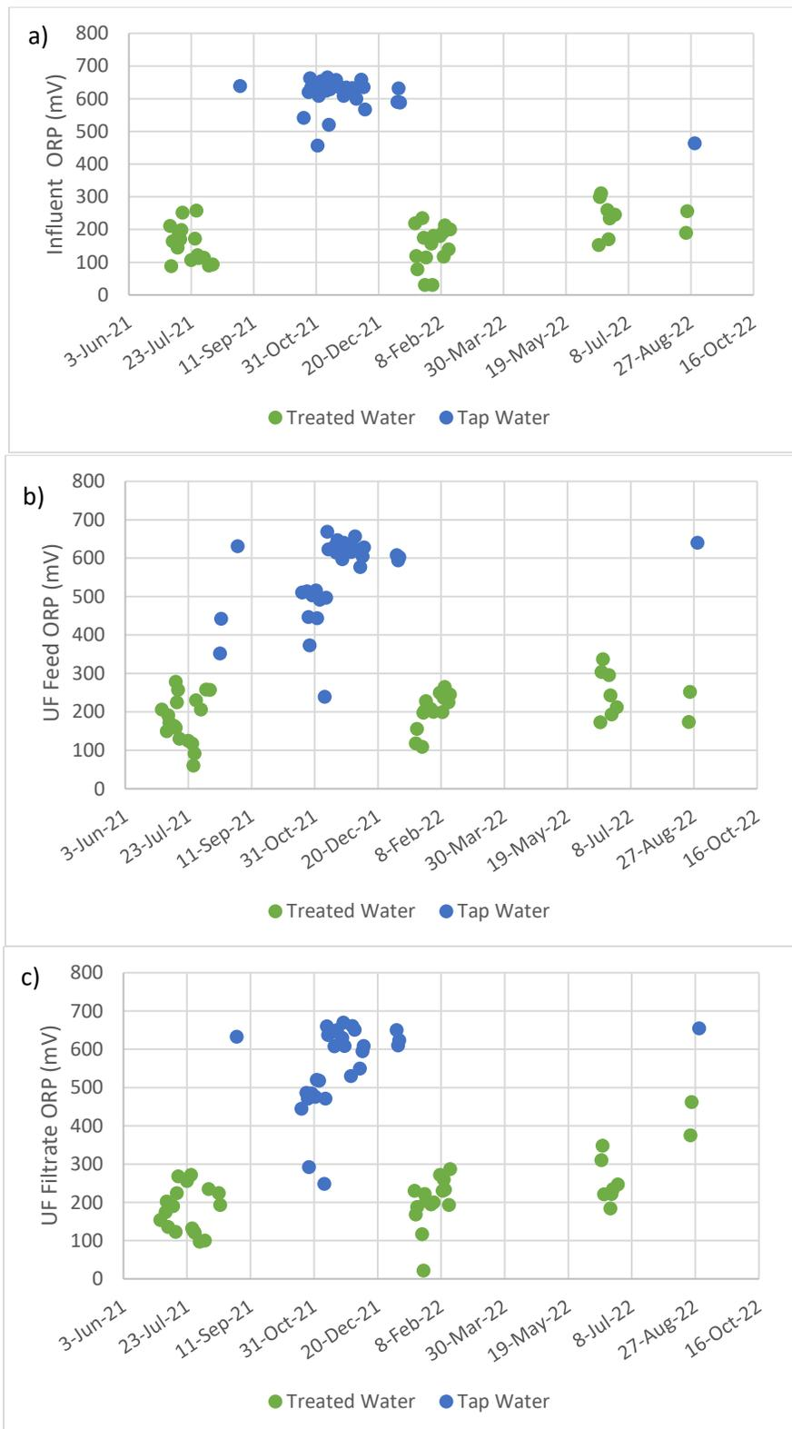
Figure 10. a) Influent ORP, b) UF Feed ORP, and c) UF Filtrate ORP (June 2021-August 2022)
