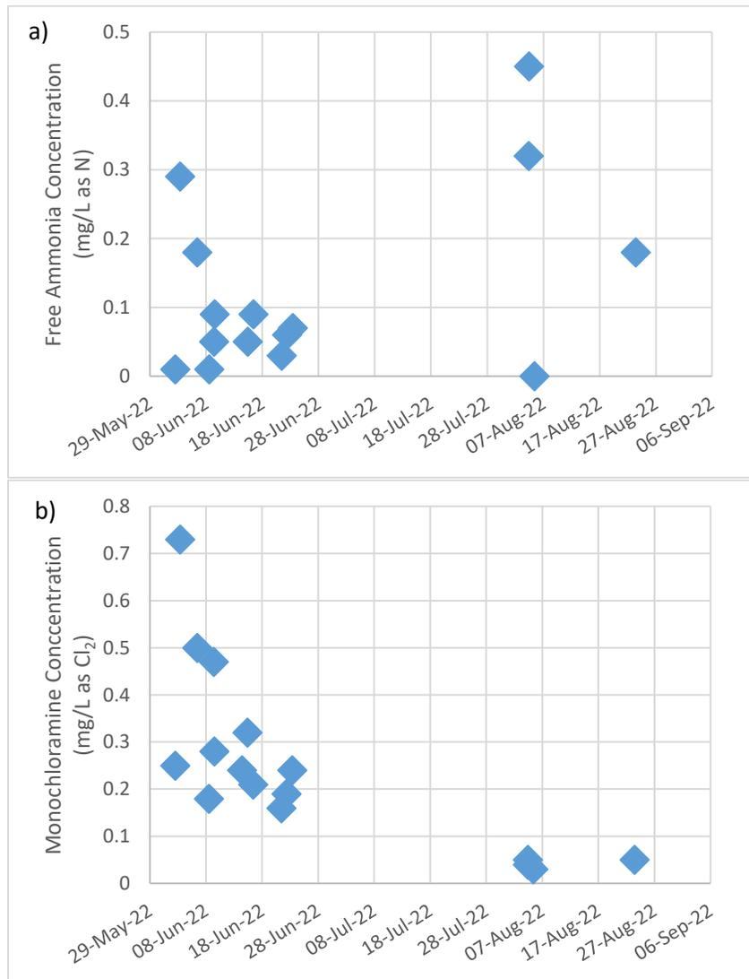
Figure 3 UF Filtrate a) Free Ammonia Concentration and b) Monochloramine Concentration at 13% LAS and 80% Bleach pump (June 2022- August 2022)
