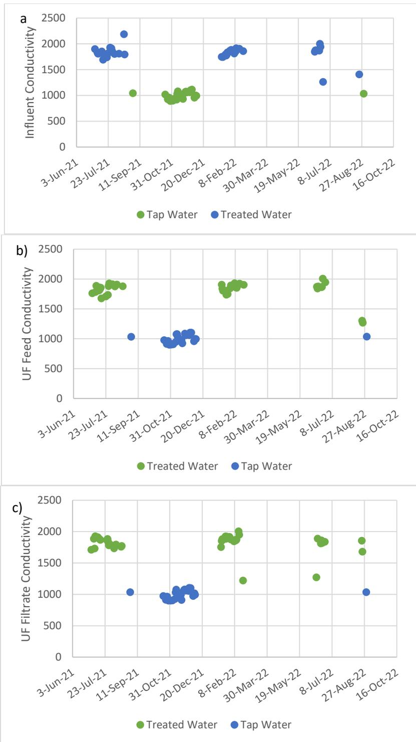
Figure 8. a) Influent Conductivity, b) UF Feed Conductivity, and c) UF Filtrate Conductivity (June 2021-August 2022)
