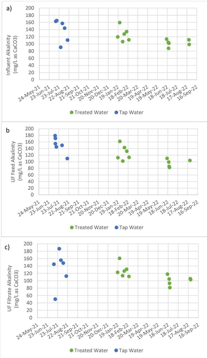
Figure 14. a) Influent Alkalinity, b) UF Feed Alkalinity, and c) UF Filtrate Alkalinity (June 2021-August 2022)
