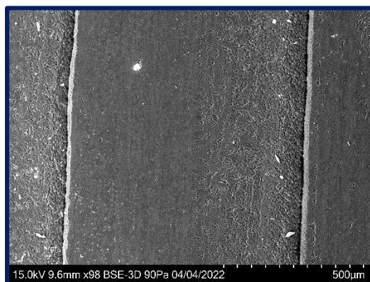
Figure 4.5 SEM micrograph for pristine SEBS:ABS extrusion
