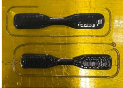
Figure 1.23: DIW Specimens with Added Milled Carbon Fiber
