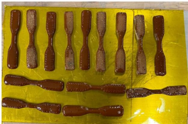
Figure 1.20: Successfully Printed Specimens
