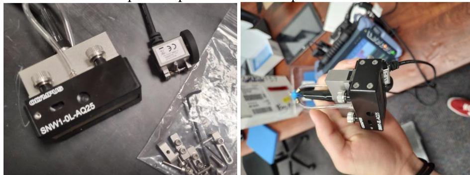
Figure 2.6: NW-1 Probe and its Components
