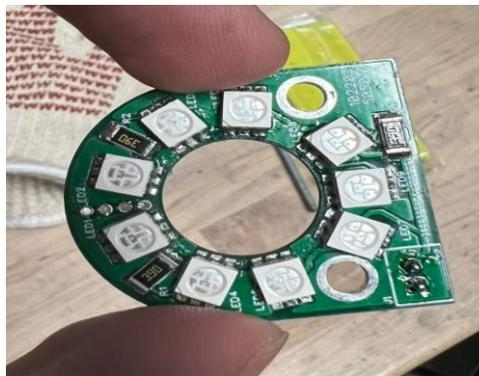
Figure 1.18: Print Head UV Array
