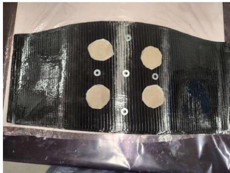
Figure 2.4: Carbon Fiber Composite Embedded Defects
