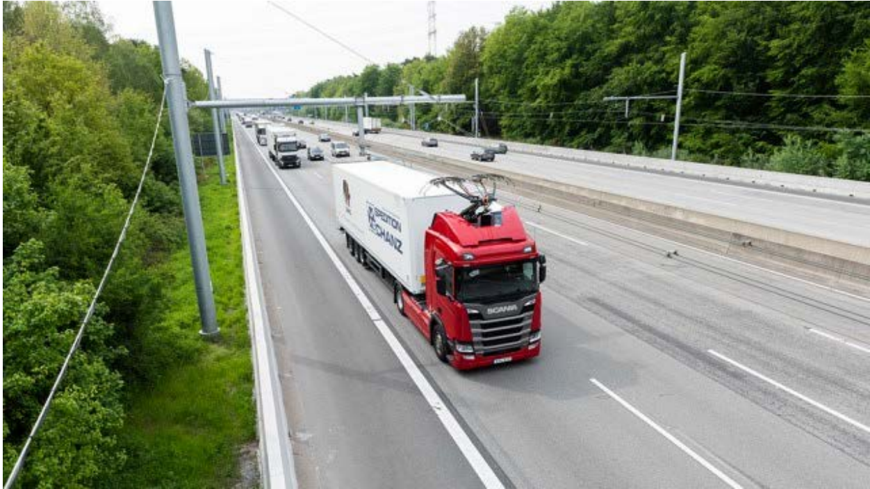
Figure 1 - Siemens First eHighway in Germany (Siemens, n.d.)
