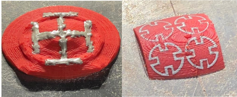
Figure 32. (Left) Jerusalem cross conformally printed on a random hill. (Right) Small array of ring loops printed on a curved surface.
