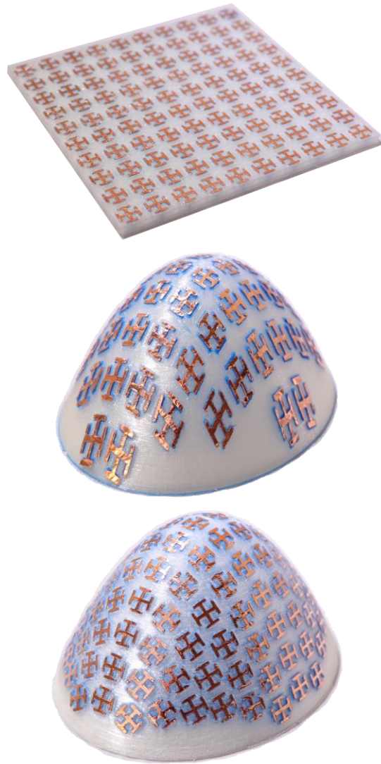
Figure 59. Manufactured FSS with Jerusalem crosses. (Top) Standard flat FSS. (Middle) Projected FSS. (Bottom) SVL tool FSS. [94]
