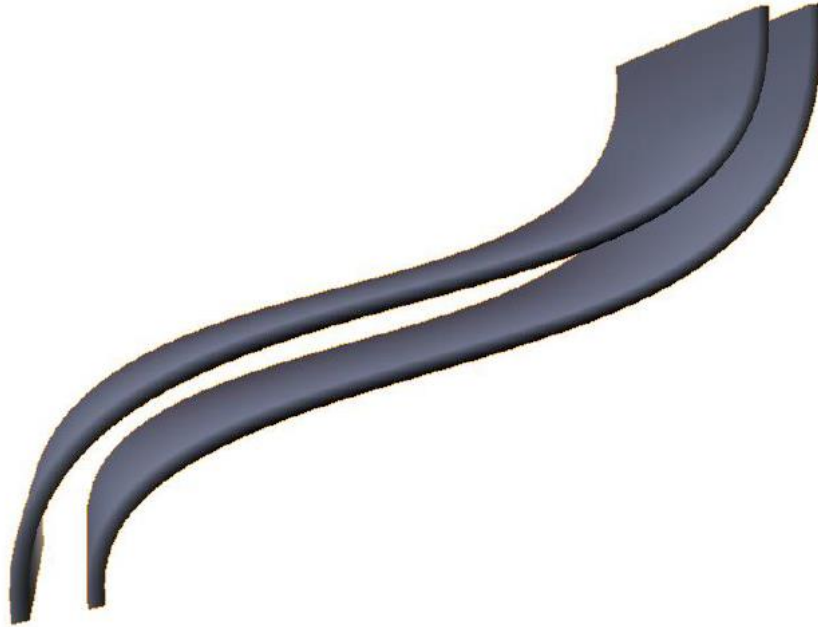
Figure 7. Rendered model of a parallel-plate transmission line.
