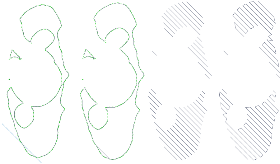
Figure 14. (Left to Right) Steps of generating infill. 1. Draw a line through the perimeter. 2. Clip the line at the perimeter. 3. Repeat until the slice has been covered. (Perimeter not shown.) 4. Stitch the lines together via the closest line segment.
