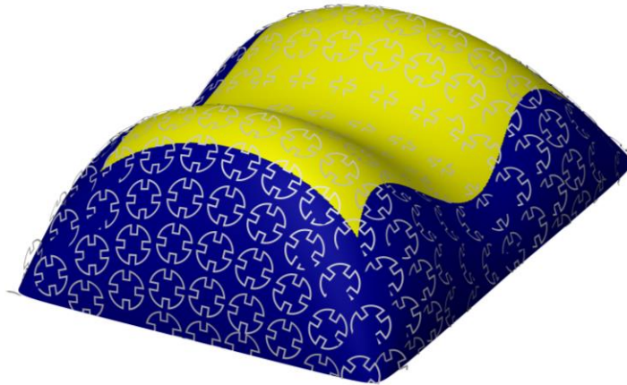
Figure 62. Regions of conformal slicing in yellow vs. steep conformal slicing in blue.
