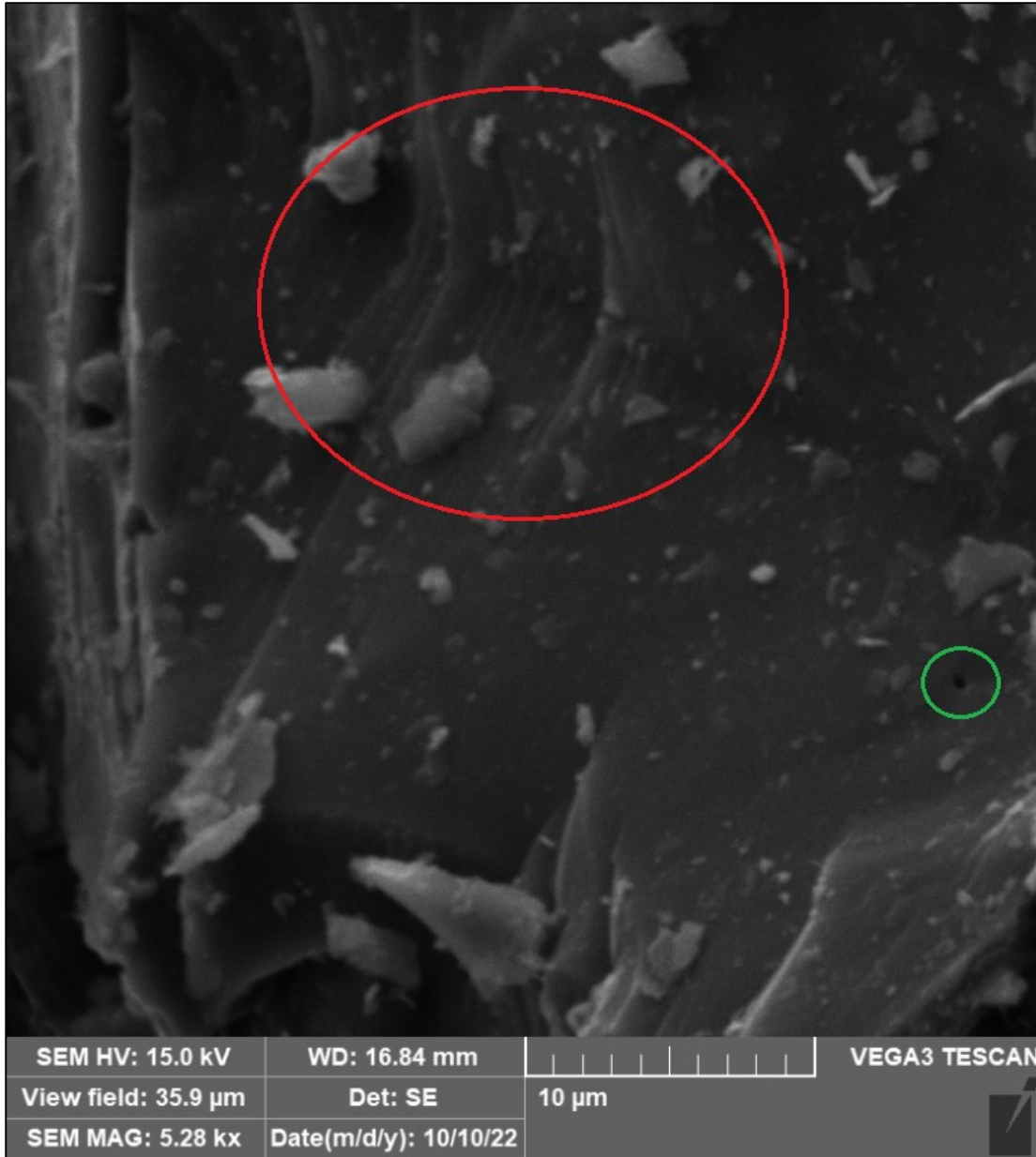
Figure 45: SEM imagery of quartz surface. Conchoidal fractures (circled red), along with an air void (circled green). Flat surfaces are relatively smooth.
