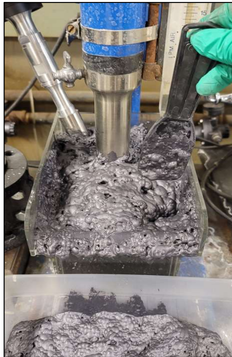
Figure 29: Image showing the paddling of 2CF froth into concentrate container.
