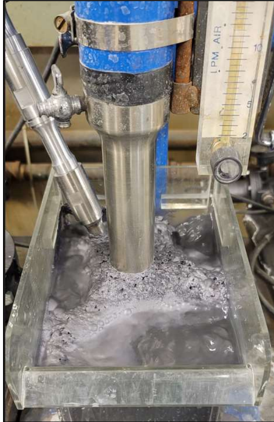
Figure 42: Probe prevents the paddle from accessing about 1.5 in 2 of float cell.
