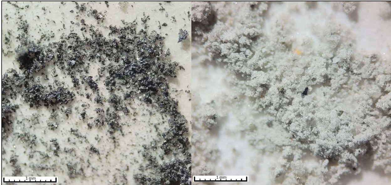
Figure 22: 2CF (left) and CRC (right) samples under an optical microscope. CRC possesses larger particle sizes and a larger percentage of gangue.
