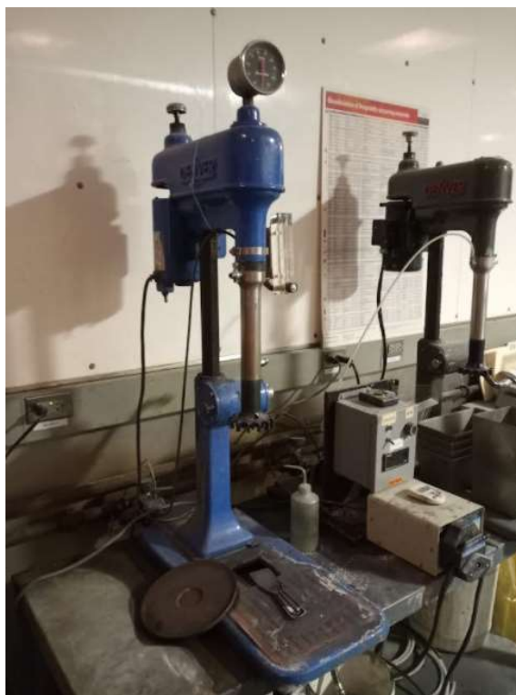
Figure 17: The Denver Cell D12 Lab Flotation machine used in these experiments.
