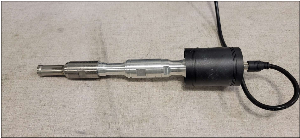
Figure 19: The 2000W 24 kHz Ultrasonic probe used in these experiments.
