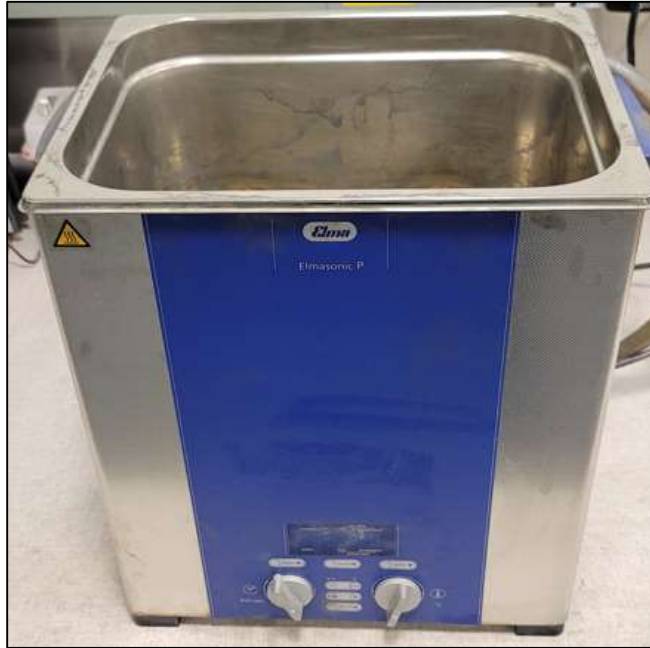
Figure 18: The ultrasonic bath used for the experiments, an Elmasonic P 120 H ultrasonic bath.
