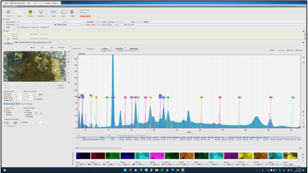
Figure 3.10: Screen image of the Bruker M4 Tornado showing spectrum collected from sample ROD-1 (green outline in Fig. 3.9, right)
