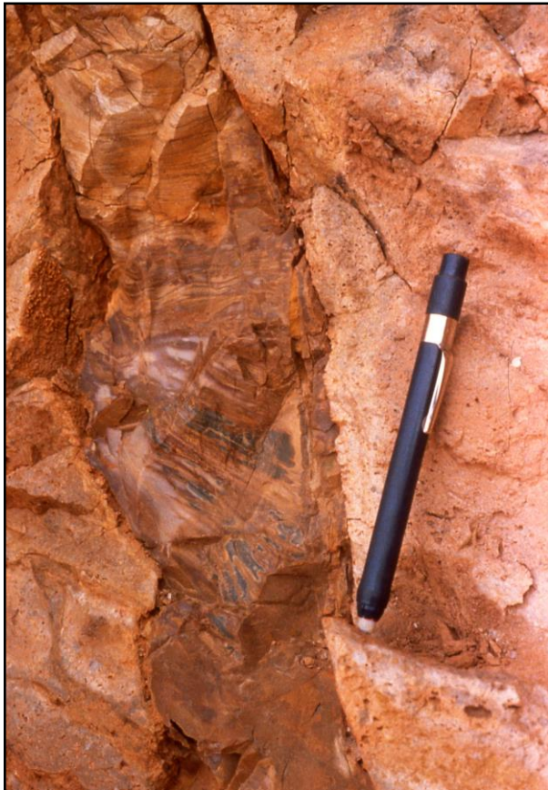
Figure 3.6: Banded chalcidonic ore at Rodalquilar: fracture filled with Au-bearing black, horizontally banded chalcidonic quartz. Some layers appear light in color due to weathering of sulfides. Average Au grade for the vein is 15 g/t; the Au content of the vuggy silica envelope is 1.3 g/t (Arribas et al. 1995).
