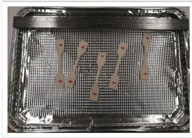
Figure 4.8 Samples moved due to mechanical recovery.
