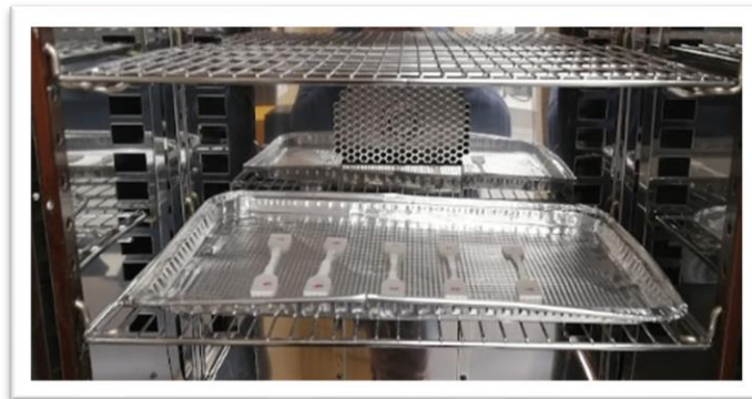
Figure 4.7 Elongated samples are set at the interior of the oven.
