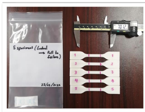
Figure 4.2 PLA-SEBS 50/50 Pull to failure (Baseline) 3D-printed samples.
