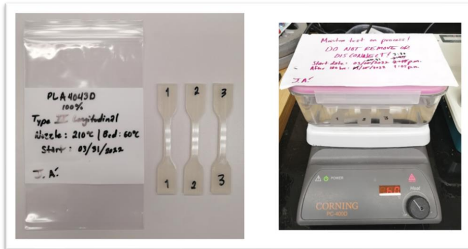
Figure 4.17 Pure PLA 3D-printed samples are set for submersion process.
