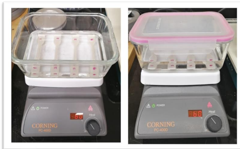
Figure 4.21 Sample submersion process.
