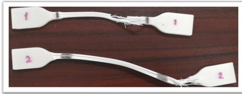
Figure 4.23 Samples 1 & 2 after being pulled to failure.
