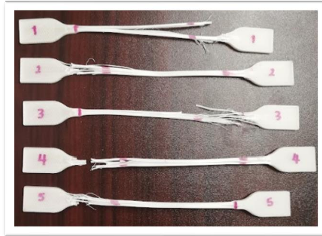
Figure 4.3 Samples after being pulled to failure.
