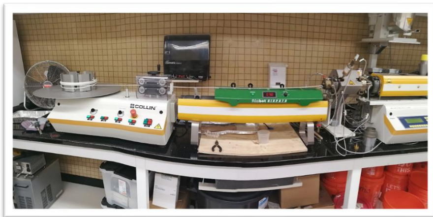
Figure 3.2 Techline ZK 25 Compounder, cooler & belt puller with filament winder stations.
