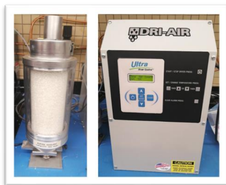
Figure 3.1 Micro Dryer CAFM (drying material equipment).
