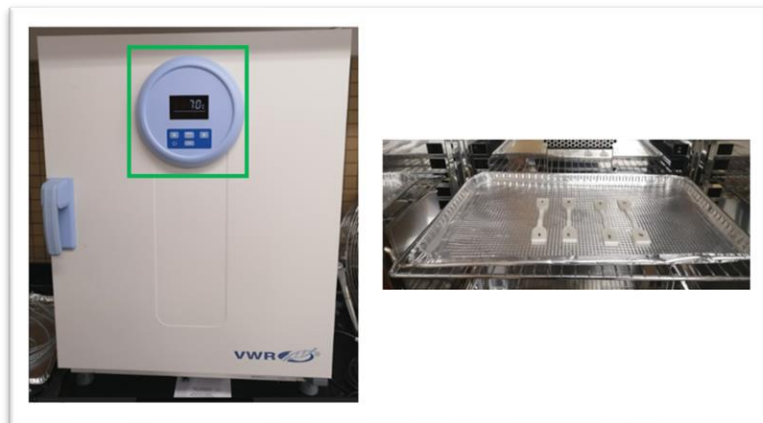
Figure 4.28 Samples set at interior of the oven at 70°C.
