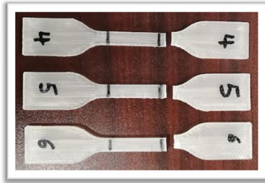
Figure 4.1 3D- Printed samples after being pulled to failure.
