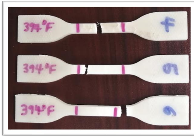
Figure 4.36 Samples after being pulled to failure.
