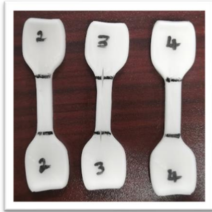
Figure 4.15 Samples set for tensile test.
