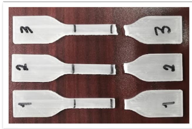
Figure 4.19 Samples after being pulled to failure.
