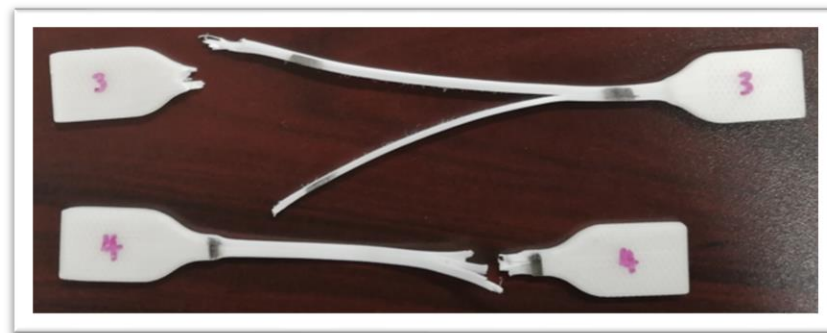
Figure 4.24 Samples 3 & 4 after being pulled to failure.
