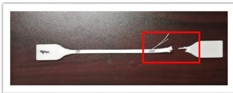
Figure 3.11 Sample No. 1 break point at 135.65 mm.
