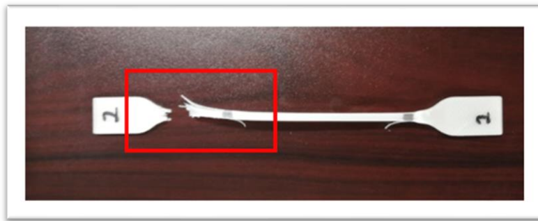
Figure 3.13 Sample No. 2 break point at 136.05 mm.
