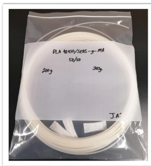
Figure 3.4 Final extruded filament.
