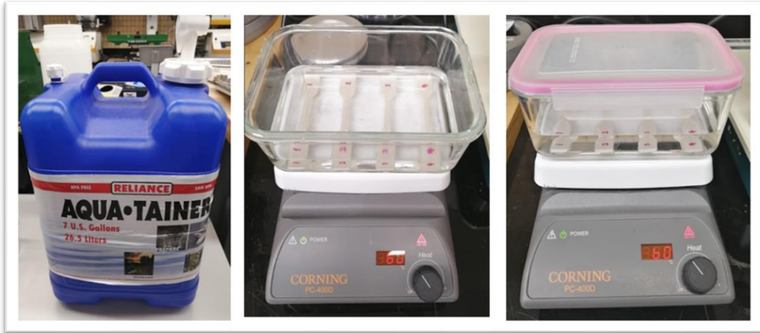
Figure 3.19 Sample submersion process.
