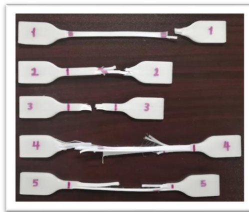
Figure 4.11 Samples after being pulled to failure.
