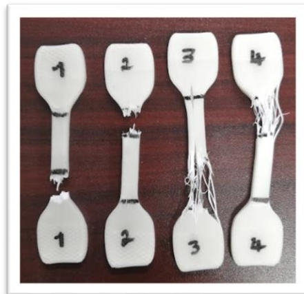
Figure 4.16 Annealed samples after being pulled to failure.
