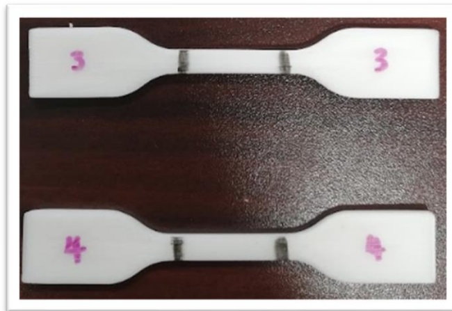
Figure 4.22 Samples prepared before tensile testing.
