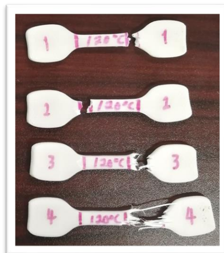
Figure 4.34 Samples after being pulled to failure.
