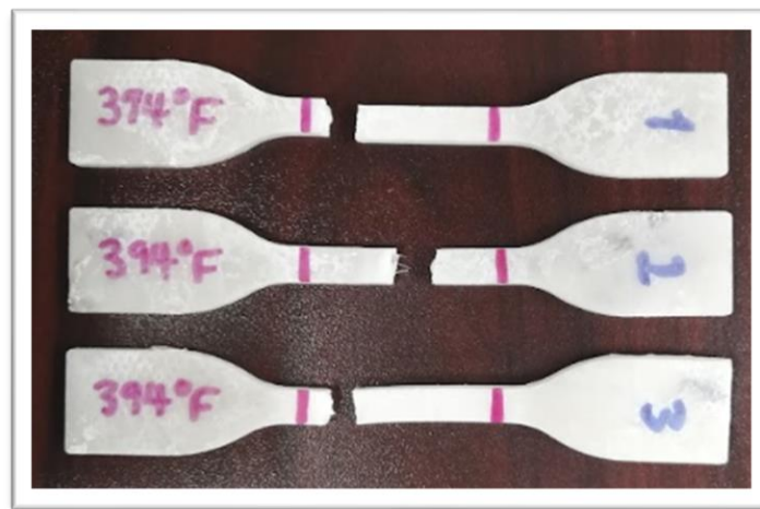
Figure 4.39 Samples after being pulled to failure.
