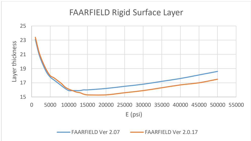
Figure 4.12: FAARFIELD Rigid Air Force Med, Base 8in, Subbase 12in, R=650
