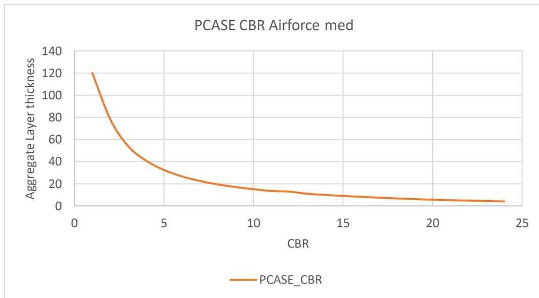
Figure 4.14: PCASE CBR Design with Airforce Med mix, Surface 4in, Stabilized base 6in
