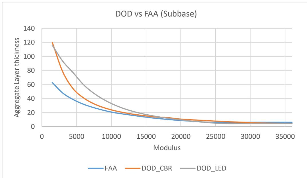
Figure 4.28: DOD vs FAA Flexible Design, Air Force Medium Mix, 4in Surface layer, 6in Stabilized Base layer
