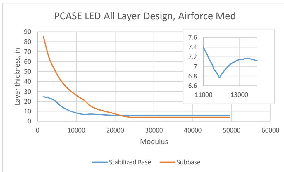
Figure 4.18: PCASE Multiple Layer Design, Airforce Medium Mix Deviation
