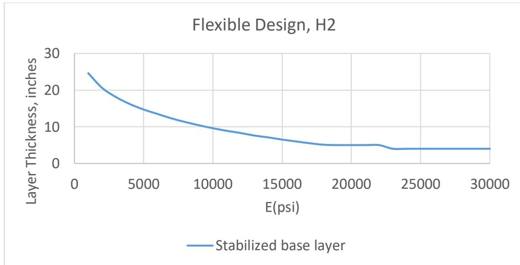
Figure 4.4: Flexible Design, Stabilized Base analyze, Example H2 Air Traffic Mix, 4-layer system
