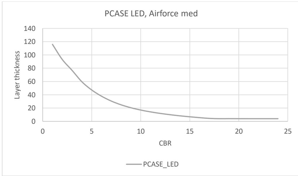
Figure 4.13: PCASE LED Design with Airforce Med mix, Surface 4in, Stabilized base 6in
