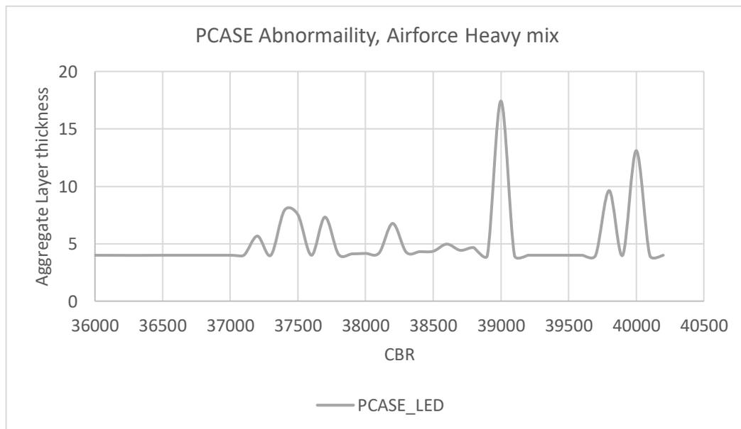
Figure 4.16: PCASE CBR Design with Airforce Heavy mix, Surface 5in, Stabilized base 6in
