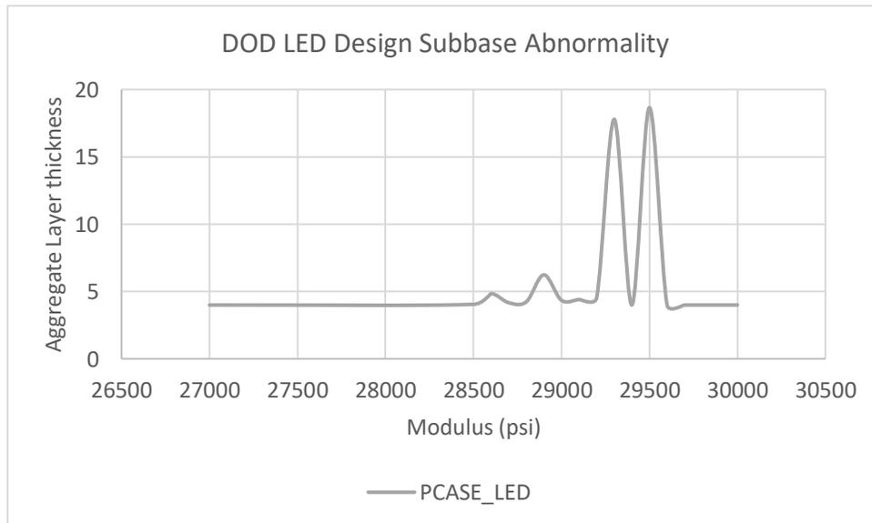
Figure 4.15: PCASE LED Design Abnormality between a modulus of 27000 and 30000 psi
