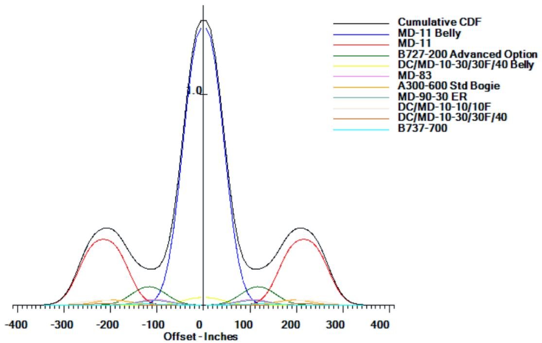
Figure 4.30: FAA CDF for El Paso Airport using Air Traffic mix from Engineer's Report
