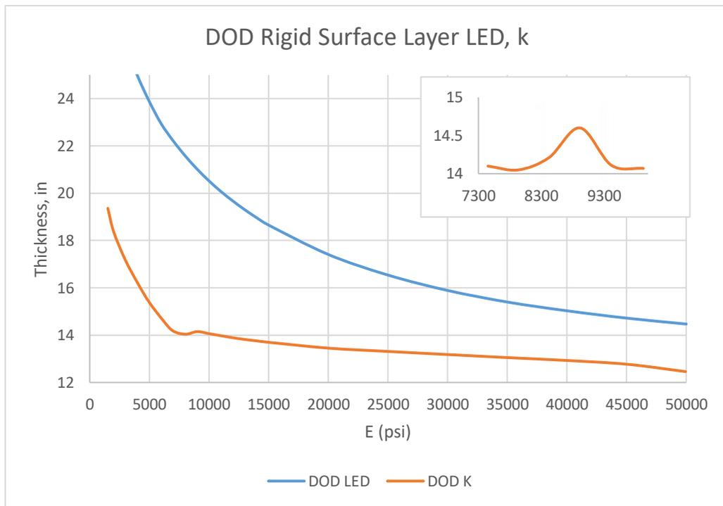
Figure 4.24: DOD LED, k Design Airforce Med, base 8in, subbase 12in
