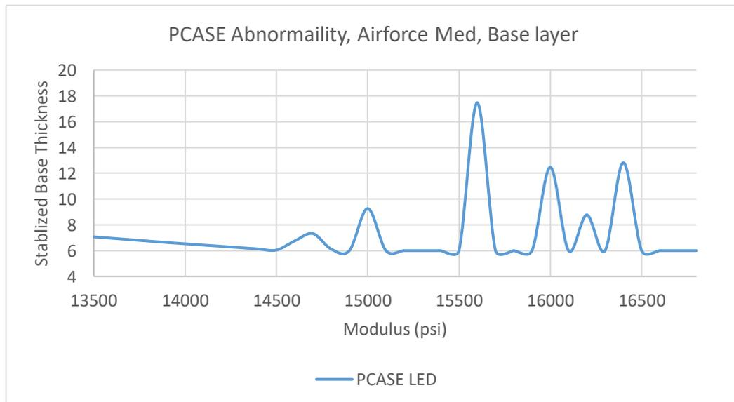
Figure 4.17: PCASE CBR Design Abnormality with Airforce Med mix, Surface 4in, Subbase 18in
