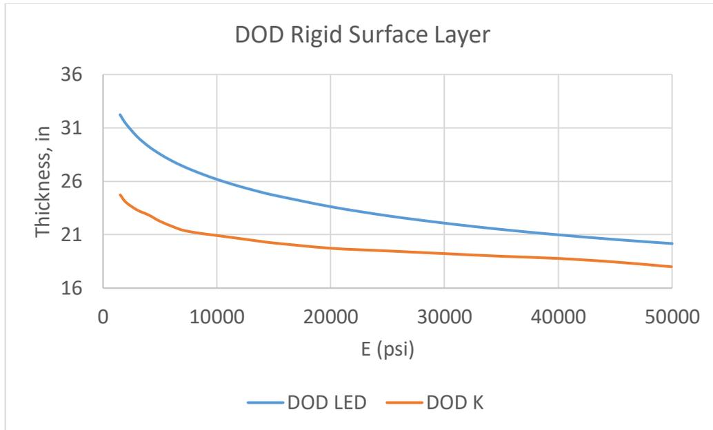
Figure 4.25: DOD LED, k Design Airforce Heavy, base 6in, subbase 12in
