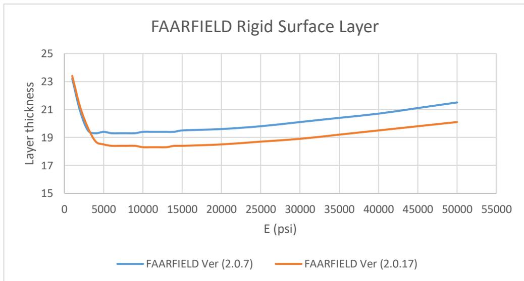
Figure 4.13: FAARFIELD Rigid Air Force Heavy, Base 6in, Subbase 12in, R=650
