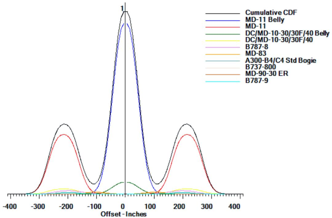
Figure 4.32: FAA CDF for El Paso Airport using Air Traffic mix from FAA for 2014-2015
