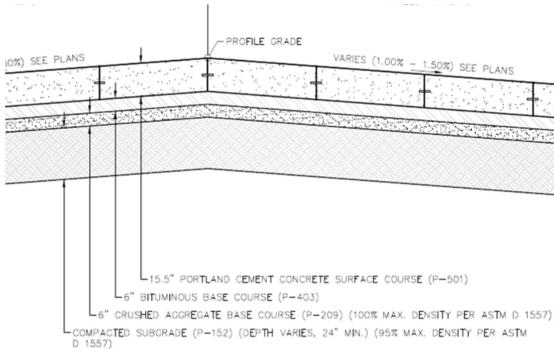
Figure 4.30: EL Paso Airport Typical Section for Runway 4-22 STA 12+20.00 to 13+00.00
