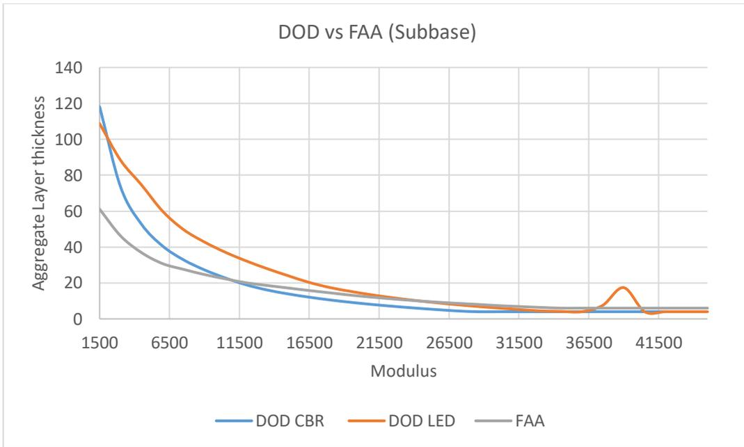
Figure 4.29: DOD vs FAA Flexible Design, Air Force Medium Mix, 4in Surface layer, 6in Stabilized Base layer
