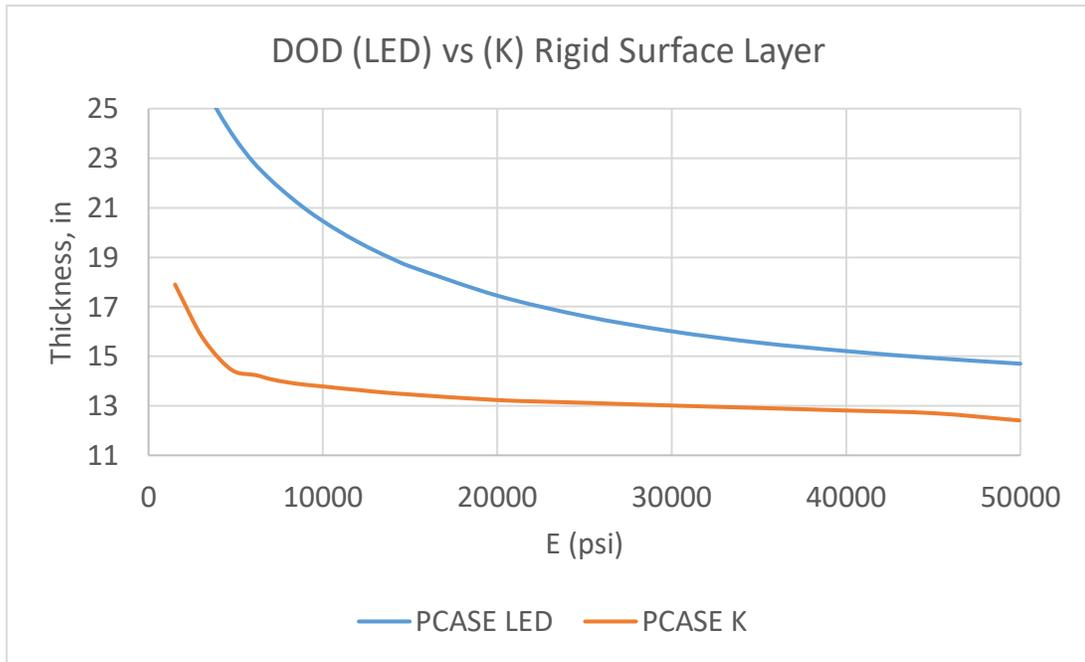
Figure 4.22: DOD LED, k Design Airforce Med, base 6in, subbase 18in
