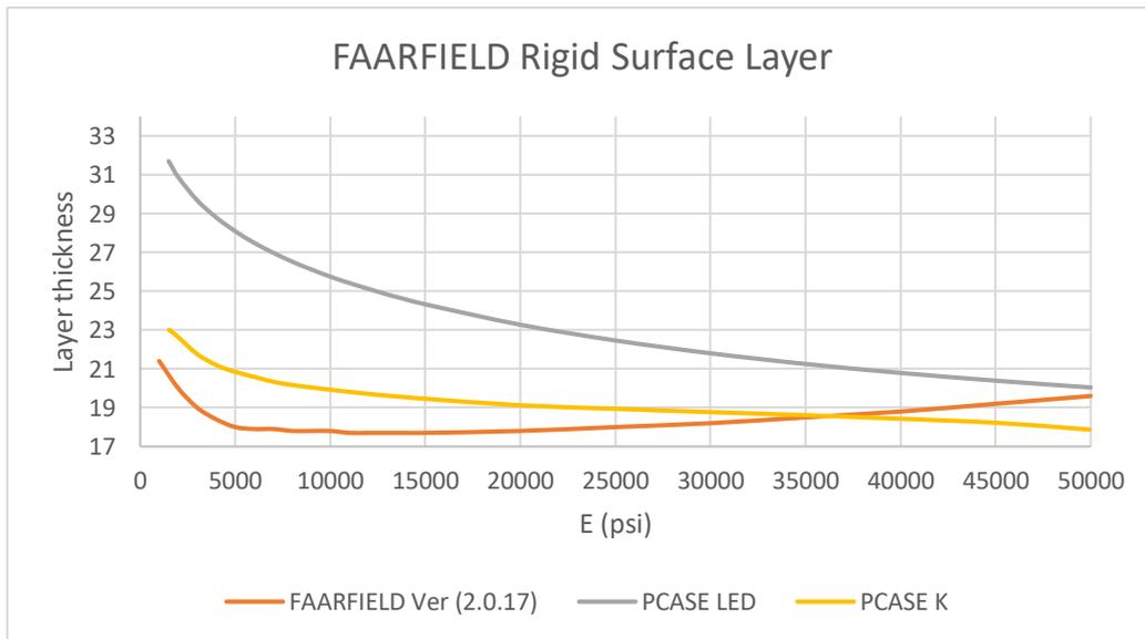
Figure 4.28: DOD vs FAA Rigid Design, Air Force Heavy Mix, 8in Stabilized base, 18 Crushed Aggregate
