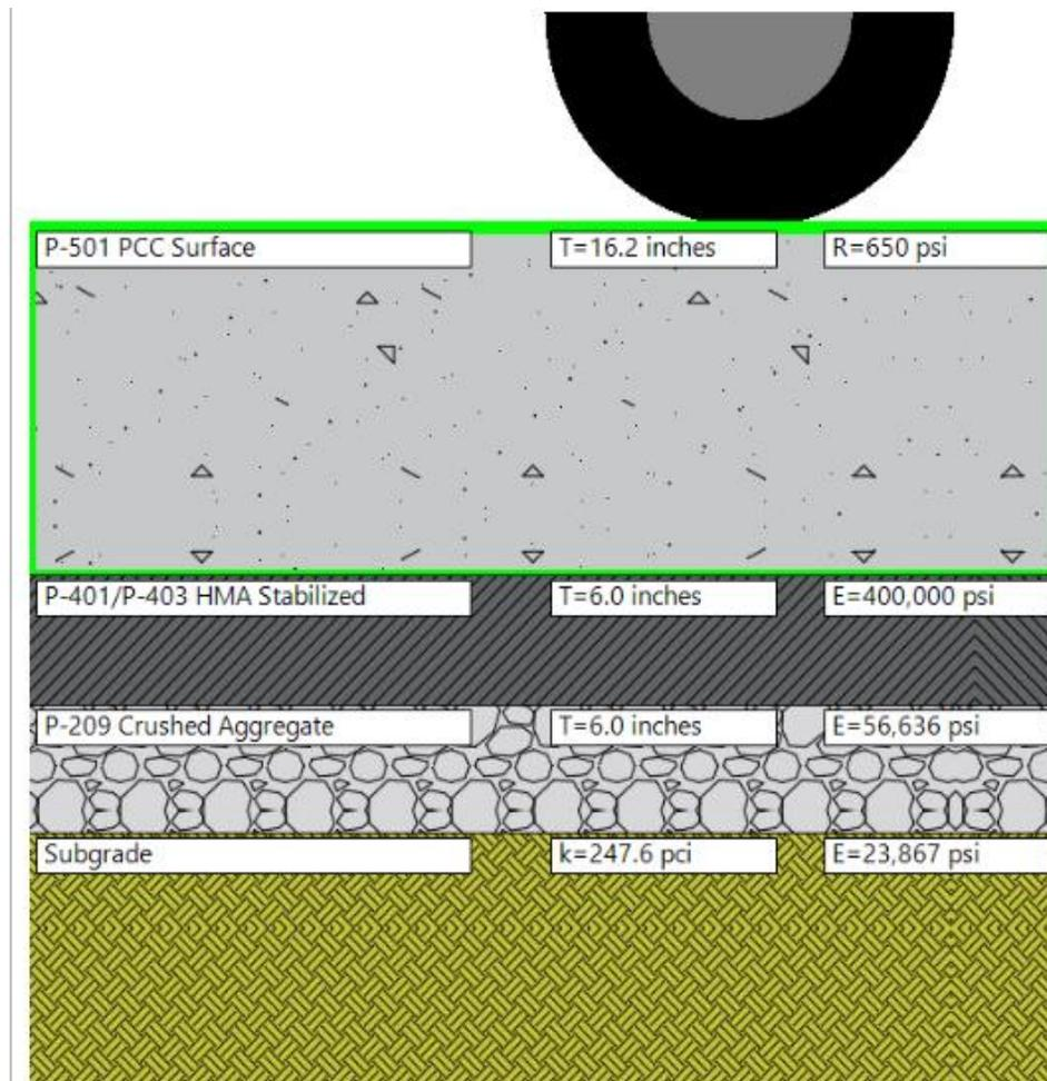
Figure 3.10: FAARFIELD Rigid pavement layer design
