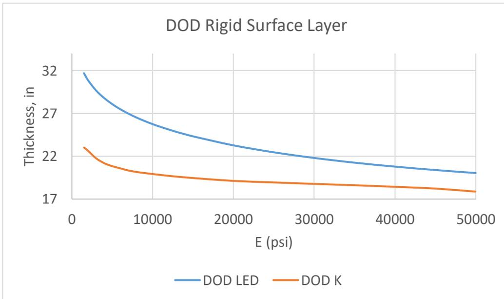
Figure 4.26: DOD LED, k Design Airforce Heavy, base 8in, subbase 18in
