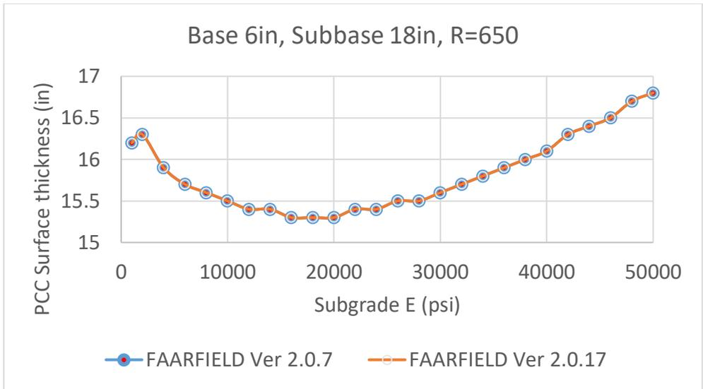
Figure 4.10: FAARFIELD Rigid Surface Layer Design under varying conditions
