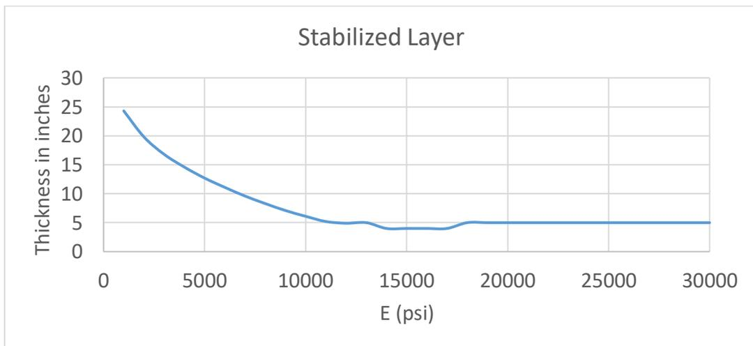
Figure 4.5: Flexible Design, Stabilized Base analyze, Example H2 Air Traffic Mix, 3-layer system
