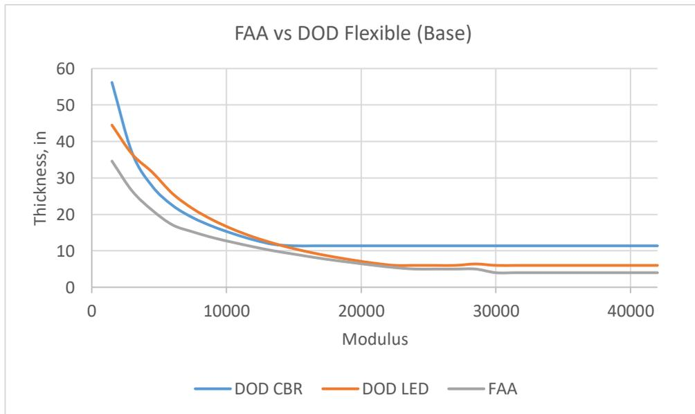
Figure 4.29: DOD vs FAA Flexible Design, Air Force Medium Mix, 5in Surface layer, 12 Subbase Base layer
