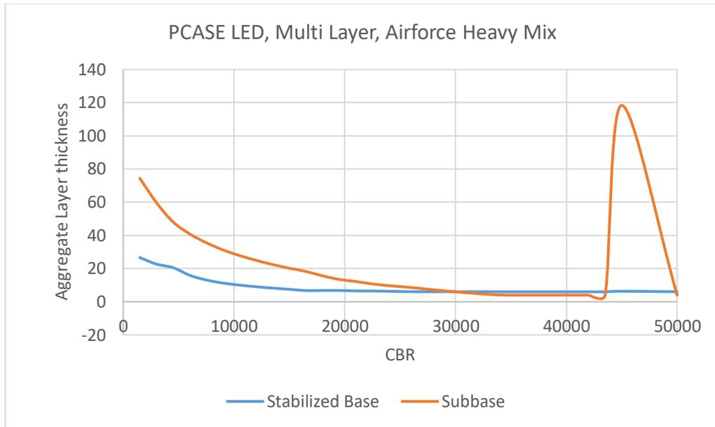
Figure 4.19: PCASE Multiple Layer Design, Airforce Heavy Mix
