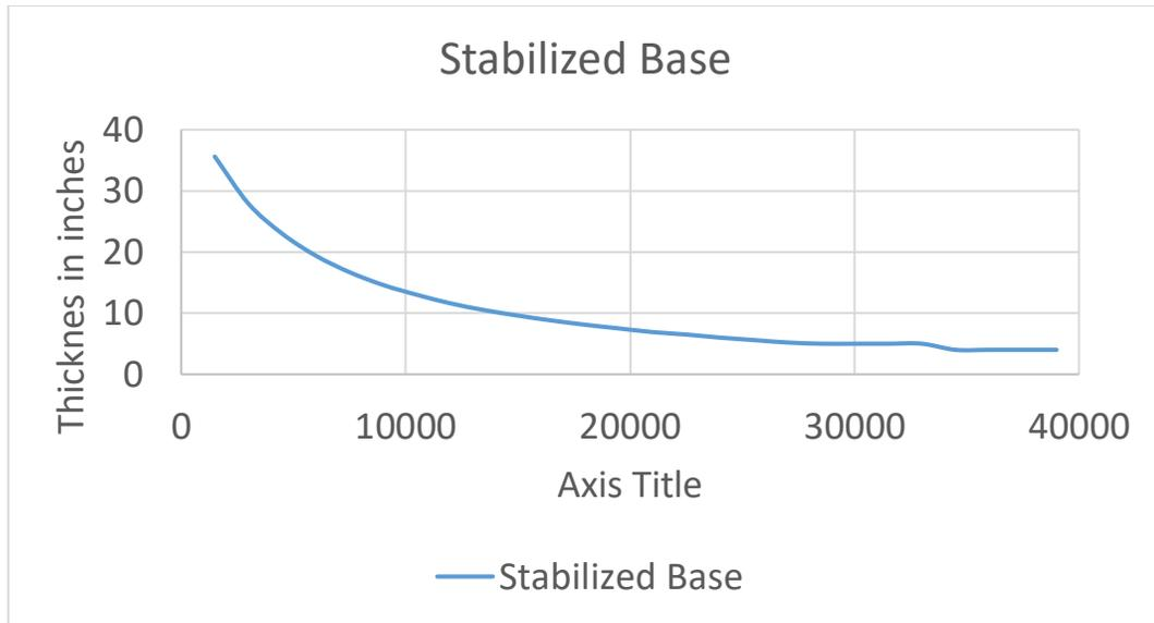
Figure 4.6: Flexible Design, Stabilized Base analyze, Airforce Medium Air Traffic Mix. 3-layer system
