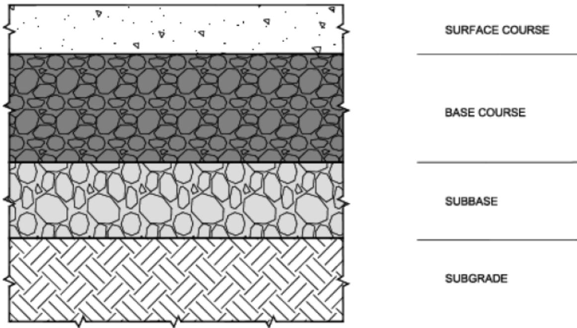
Figure 3.5: Typical Pavement structure (AC150/5320-6F)
