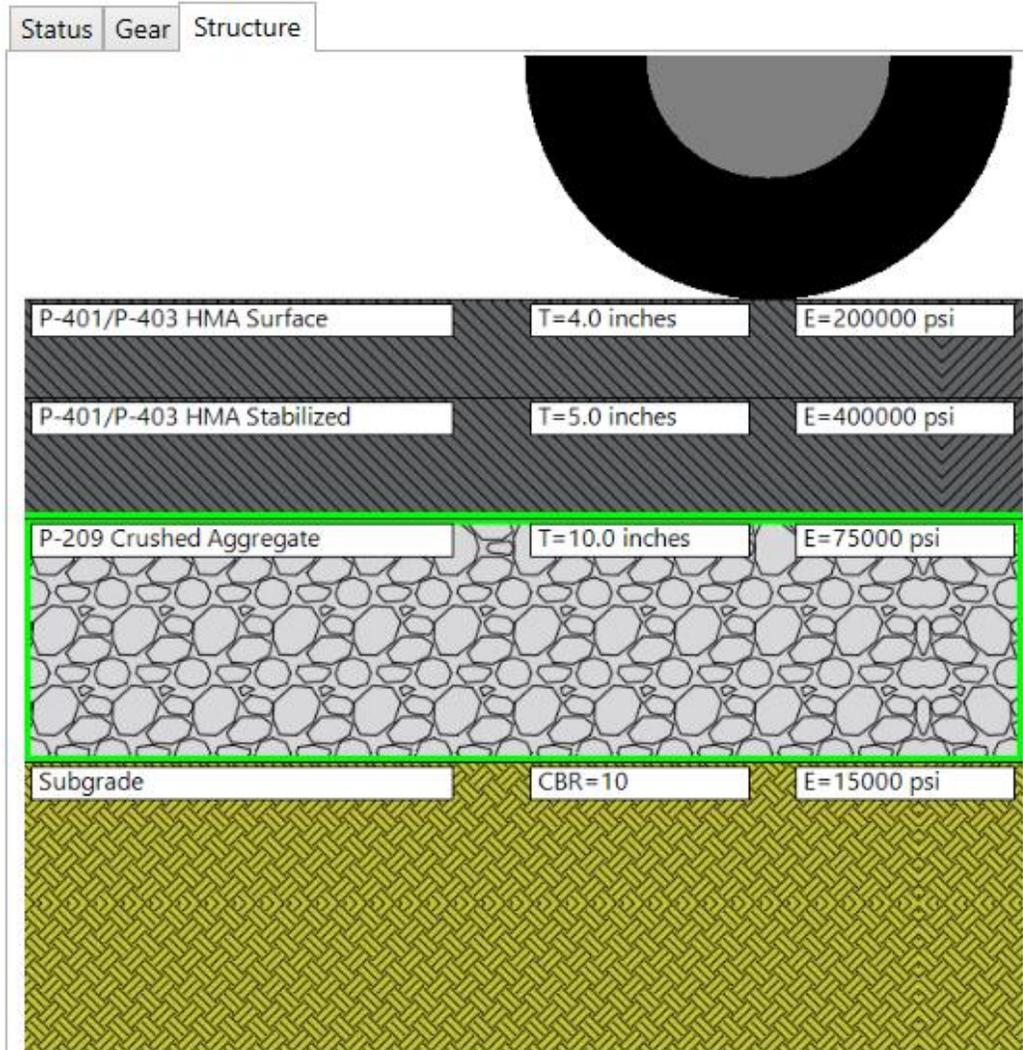
Figure 3.6: FAARFIELD Flexible pavement layer design
