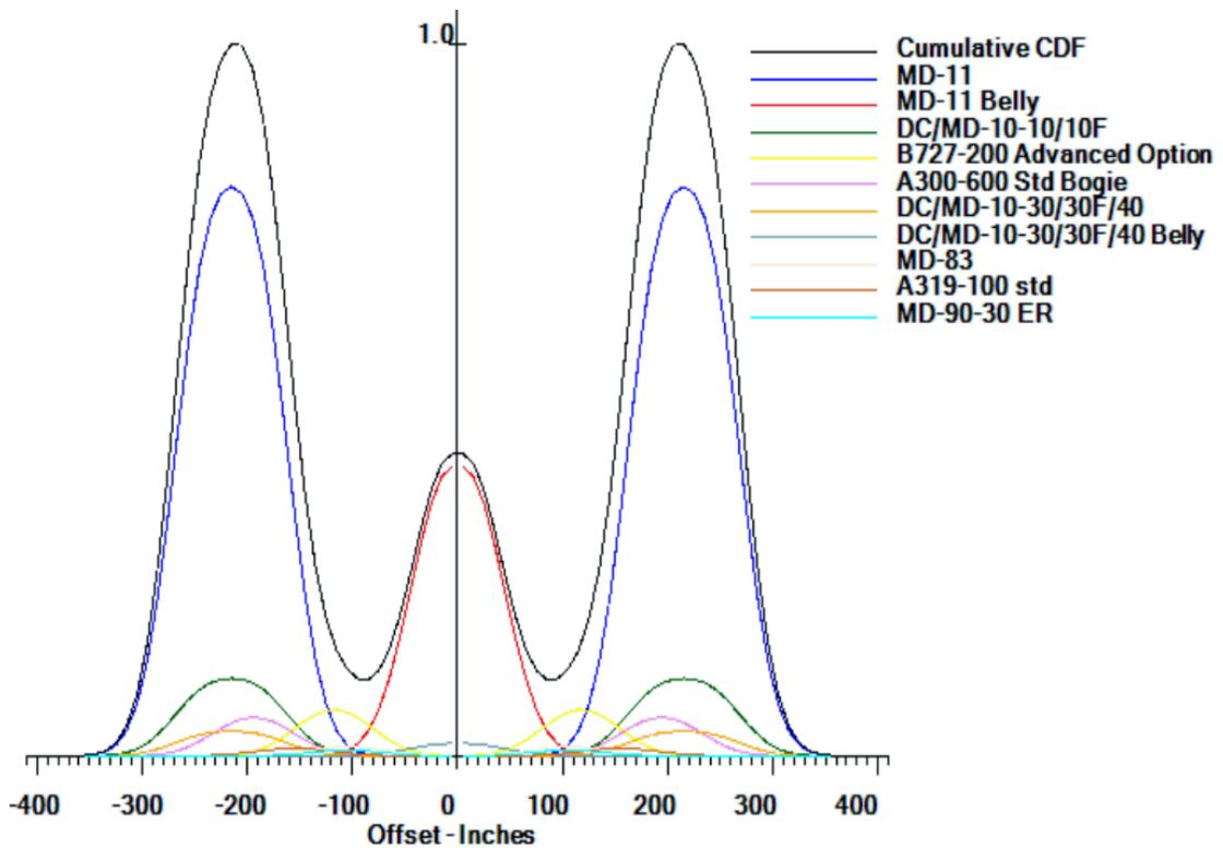
Figure 4.31: FAA CDF for El Paso Airport using Air Traffic mix from Engineer's Report with modified base and subbase
