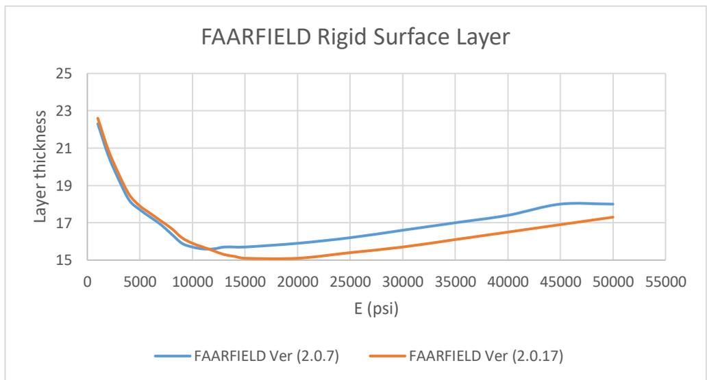
Figure 4.11: FAARFIELD Rigid Air Force Med, Base 6in, Subbase 18in, R=650
